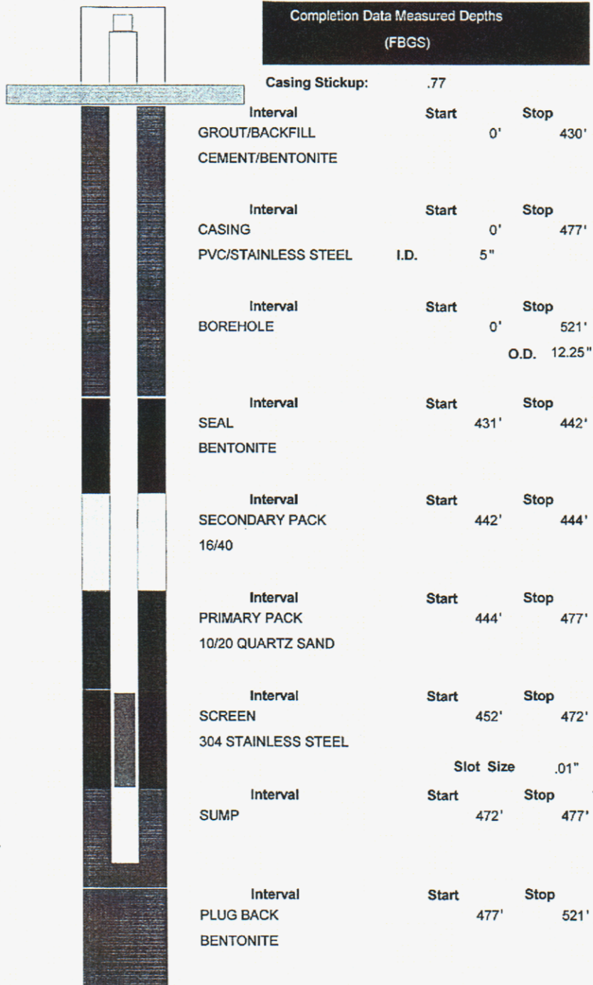
Figure 5.2-3 Well Completion Diagram for MW-2
