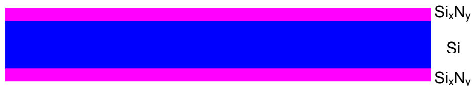
Figure 13. LPCVD silicon nitride wafer. Because the nitride serves as a hard-mask for the KOH etch, it must be deposited on both sides of the wafer.
