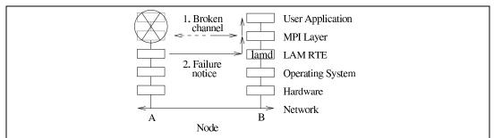
Figure 8: A user MPI process on node A has failed. If supported, the communications channel on node B will notify the MPI layer that its peer on node A has unexpectedly shut down. The lamd on A will notice that the application has failed, and send a failure notice to the lamd on B, which will be propagated up to the MPI layer. The user application may also choose to receive the asynchronous failure notices (but from the MPI layer, not from the run-time environment directly).
