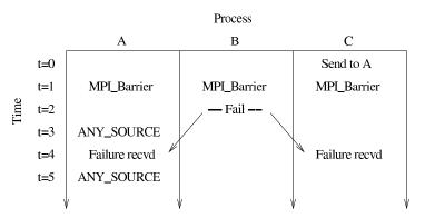
Figure 13: Timeline showing possible behavior of MPLRECV with MPLANY\_SOURCE in the presence of failures.
