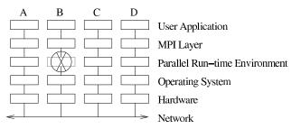
Figure 3: A parallel user application running on four nodes. Although node B itself does not fail, the run-time environment fails on B, which will propagate up to the user application and cause it to fail as well.
