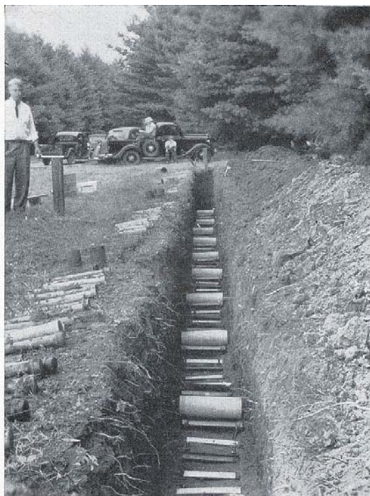
FIGURE 6.—Arrangement of specimens buried near Baltimore, Md., in 1932.
