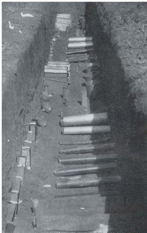
FIGURE 5.—Arrangement of specimens buried in 1924 Note two soil horizons.
