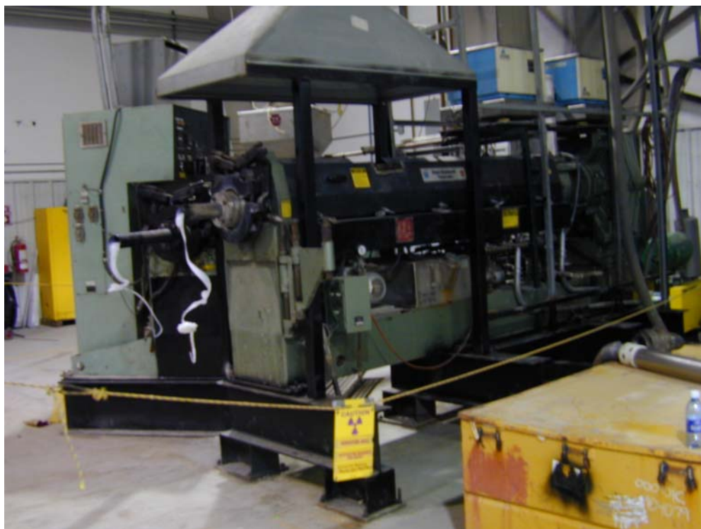
Figure 2. Polyethylene extrusion system used to process DU/poly shield
