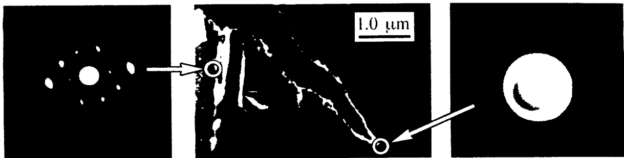
Fig. 2. Dark-field image and selected area diffraction patterns showing amorphous phase formation in the region ahead of crack tip and along the crack edges.
