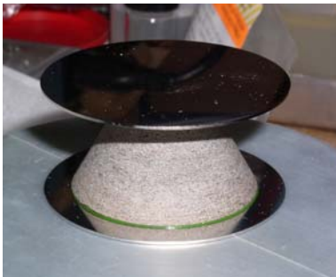
Figure 6: Mycalex cone glued to "disposable" stainless steel disks.
