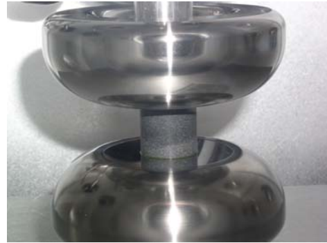
Figure 7: Mycalex cylinder between test electrodes.
