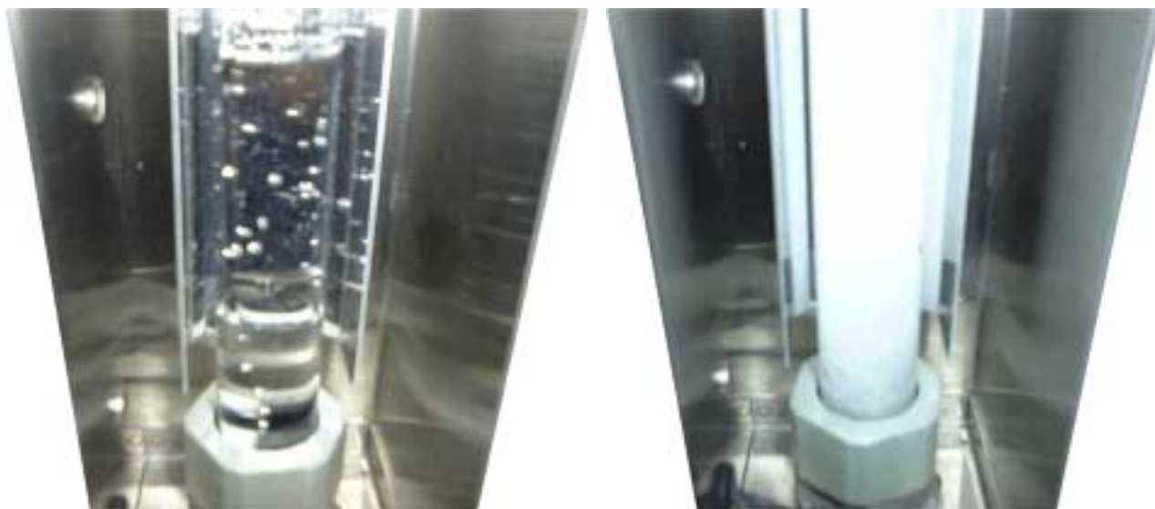
Fig. 3. Gas injection in the UV-ozonation reactor. Left: using a sparger (without electrostatic spraying); right: using a fine bubble diffuser.
