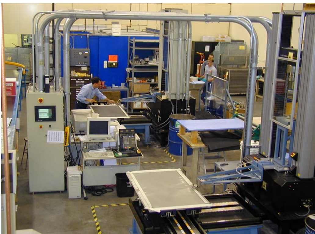
Figure 10. IMPROVED CATALYST CORRUGATION LOADING: 2 of 3 Setups for Loading Extruded DIR Catalyst into Anode Corrugations
