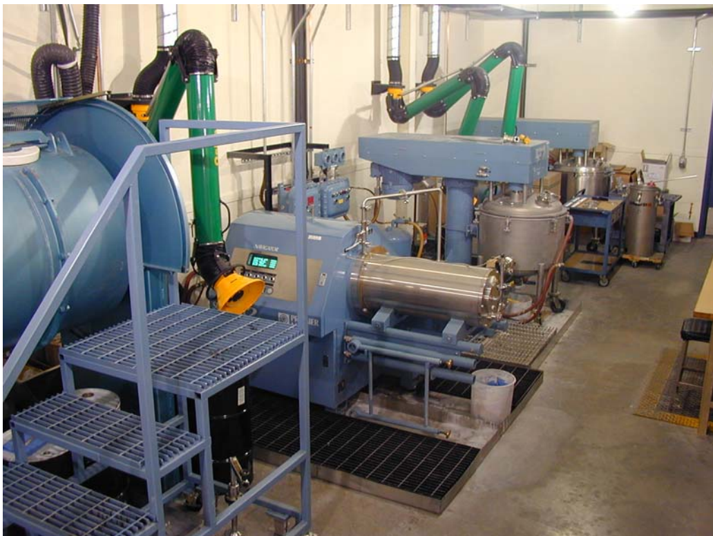
Figure 9. HIGH VOLUME SLURRY PREPARATION EQUIPMENT: Utilizes Large Mechanical Mills and Mixers
