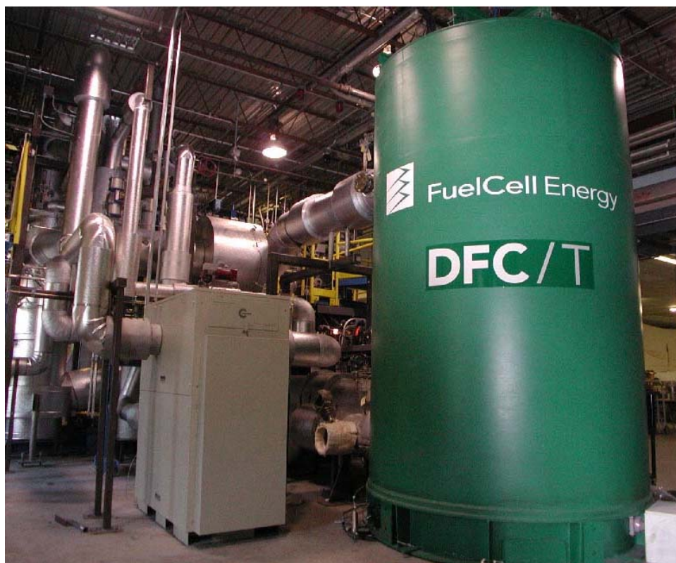
Figure 6. STACK FA-100-2 TEST IN 400 kW-CLASS POWER PLANT: DFC/T Proof-of-Concept Demonstration
