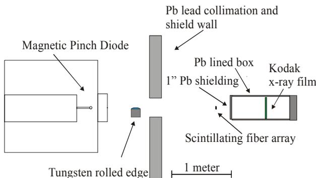
**Figure 3.** Sketch of experimental configuration.
