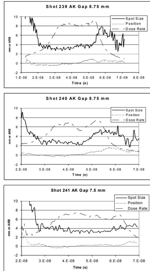
**Figure 6.** Spot size, position, and dose rate data extracted from TSRD.
