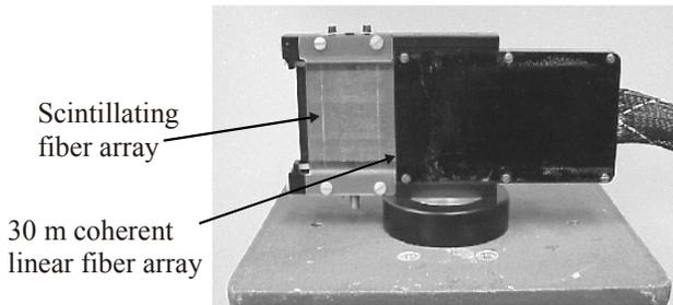
**Figure 2.** Photograph of scintillating fiber array.
