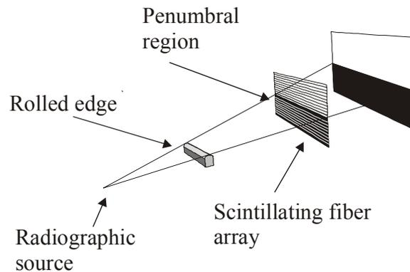
**Figure 1.** Conceptual sketch of detector array.
