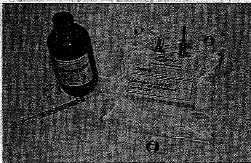
Figure 1. Tedlar Bags Used to Spike TAN Site Groundwater with Target VOCs.
