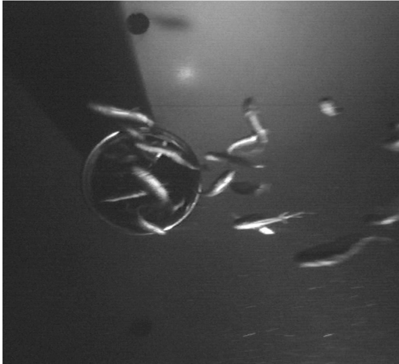
FIGURE 5-3 TREATMENT FISH EXITING INJECTION RELEASE PIPE (175 MM FISH TESTED AT A HEAD OF 38 FT)
