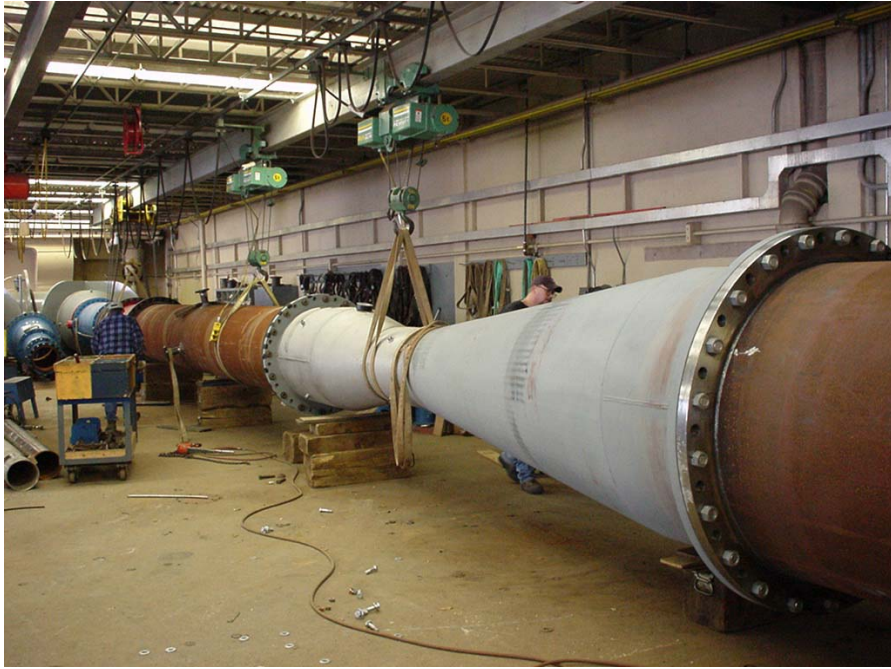
FIGURE 4-1 FLOW METER STRAIGHT PIPE CALIBRATION LOOP
