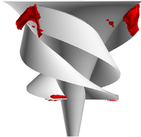
FIGURE 7-6 CLOUDS FOR NEGATIVE PRESSURE CHANGE RATE EXCEEDING -500 PSI/SEC (CASE NO. 2, 18.2^\circ WICKET GATE ANGLE FROM FULL CLOSED)
