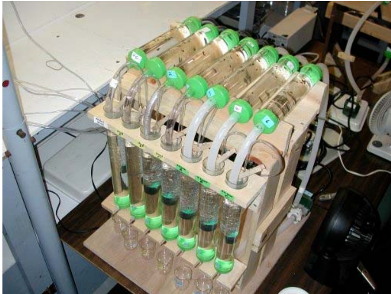
Fig. 1. Seven clear acrylic pipes with zebra mussels are an integral part of the recirculating pipe system. Each pipe has a pump and connecting hoses.
