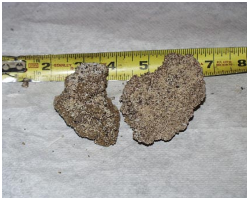
Figure 3. EXAMPLE OF CLINKERS FORMED IN FLUIDIZED BED DURING POULTRY LITTER TESTING
