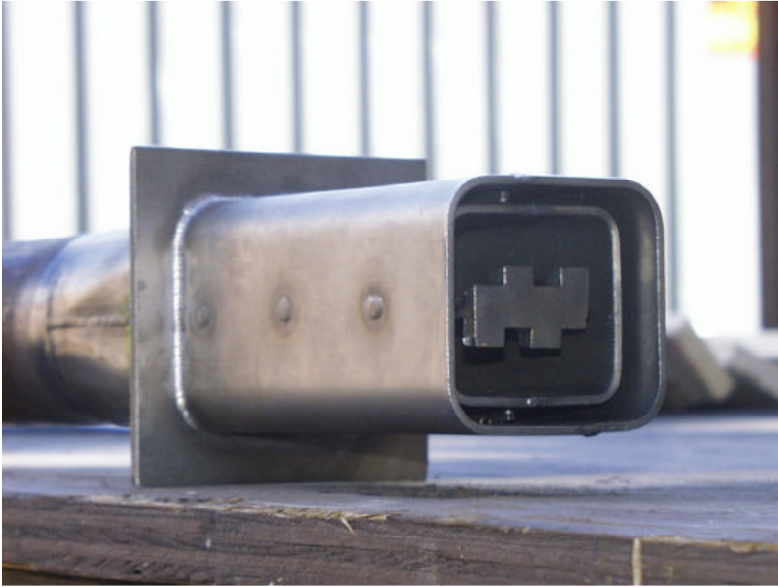
Figure 6.3-1: Photo of Coal Nozzle Tip Used During BSF Testing.
