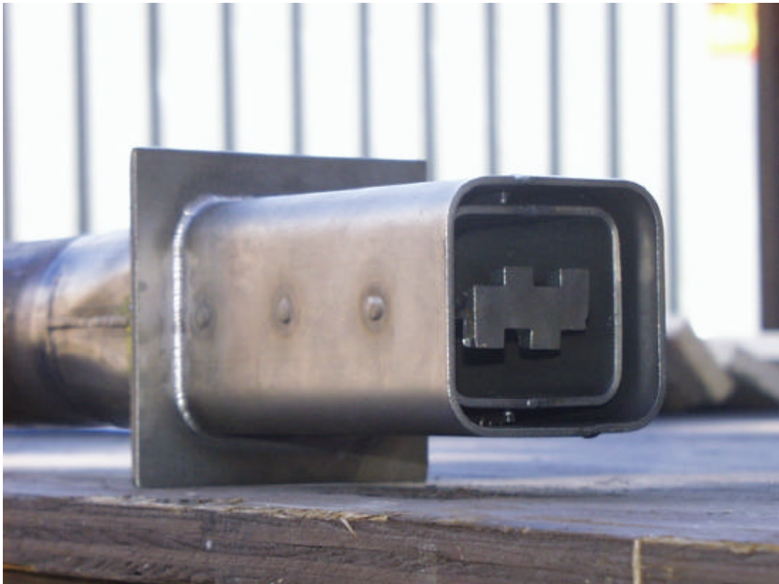
Figure 5.3-3: Photo of the Oxidative Pyrolysis Coal Nozzle Tip Used in BSF Testing.
