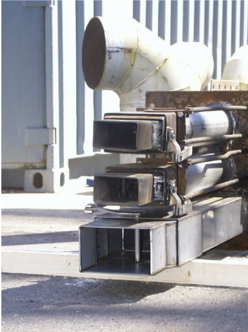
Figure 6.3-3: Photo of Modified SOFA Assemblies Used During BSF Testing.
