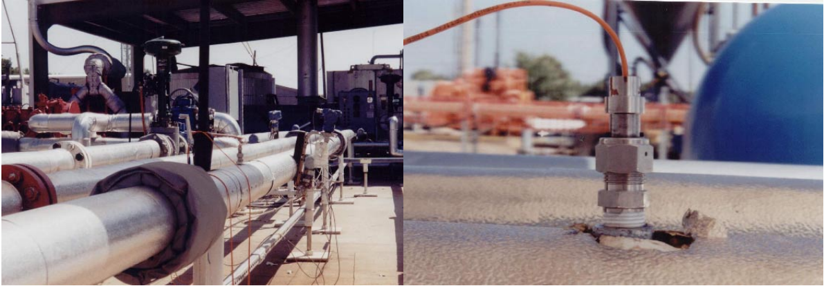
Figure 4.9. Fiber optic flow sensor deployment in outdoor flow loops of Tulsa University, OK.
