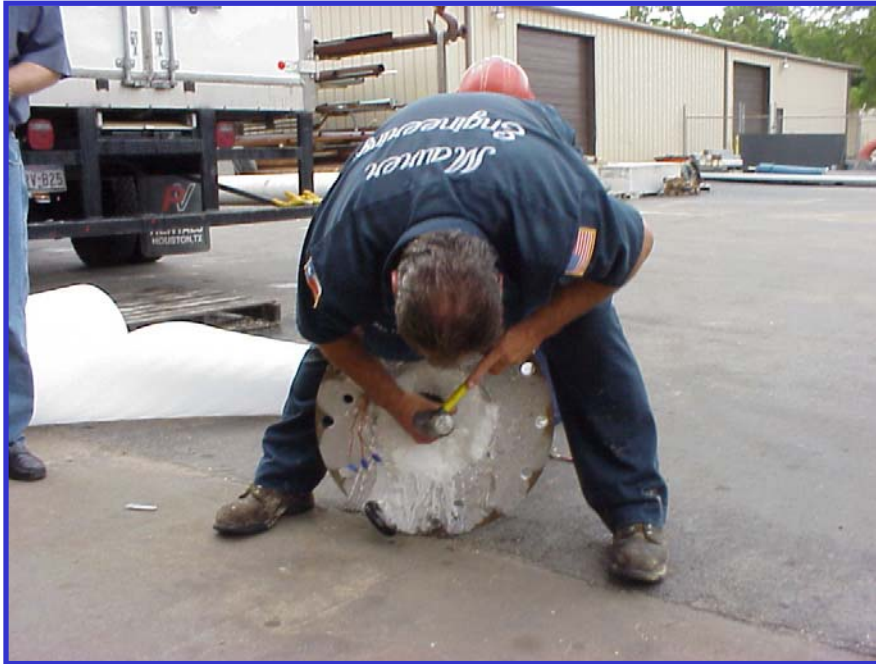
Figure 28: Frozen Core Preparation Before Coring Operation (Cont'd)
