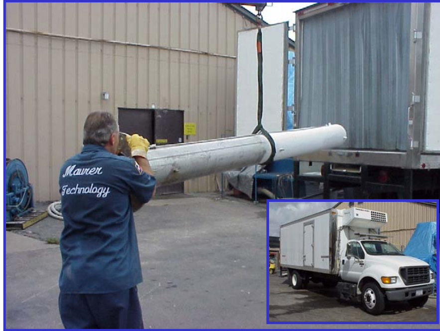
Figure 18: Bringing Core #1 from the Core Apparatus to the Freezing Truck (Cont'd)
