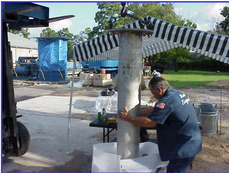
Figure 7: Core Placement in the Freezing Cased Well
