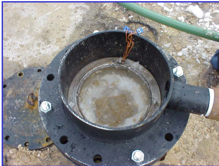
Figure 31: Frozen Core in Place to Be Cored
