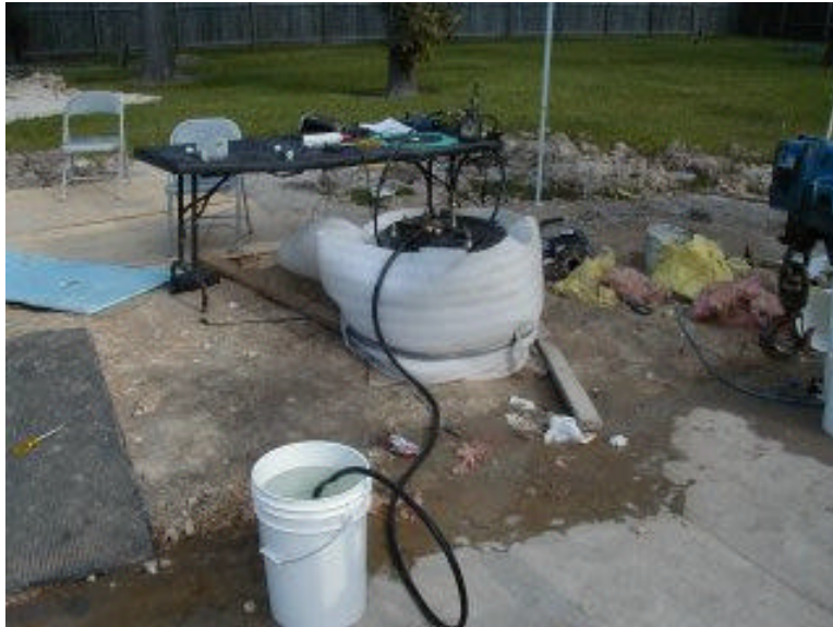
Figure 8. Vacuum Filling Freezing Chamber
