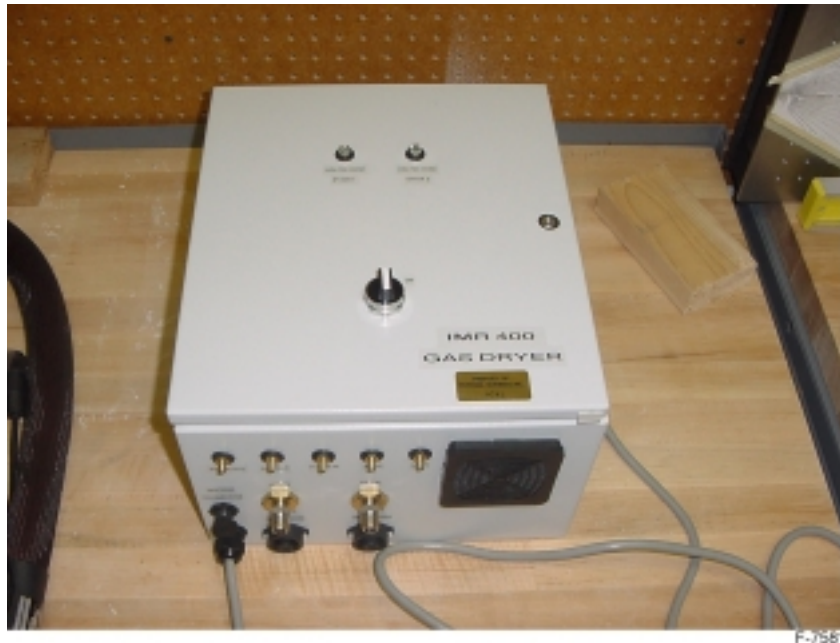
Figure 16. IMR 400 gas dryer main box.
