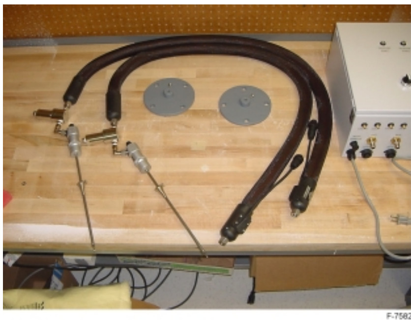
Figure 17. Gas sample hoses, probes and flanges.
