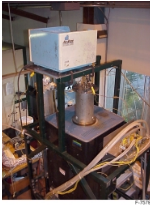
Figure 13. Coal feeder located at the top of the coal reactor.
