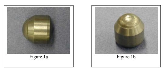
Figure 1. Two Views of the Round Top Drill Bit Insert. The insert is typical of the cutting tools placed on rotary drill bits. (Orientation of the fibrous monolith was right to left, from the round top to the flat base.)
