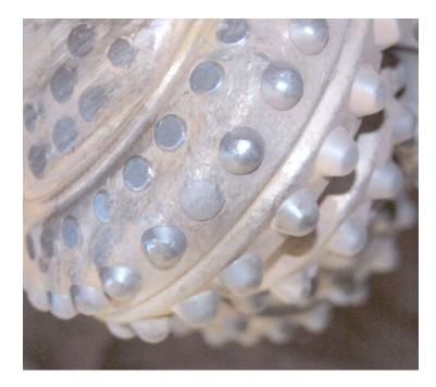
Figure 5. Current Art and Fibrous Monolith Inserts on a Worn Superior Rock Bit. The FM insert in the center has worn more than the current art inserts, although no brittle failures have occurred like the small chip on the insert to the left of the test insert.
