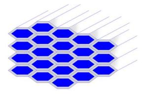
Figure 2. Schematic Drawing of the Core and Boundary Areas in a Fibrous Monolith. The test inserts were composed of a tungsten carbide core (blue, 96 % carbide) and a cobalt boundary (gray, 100% cobalt).
