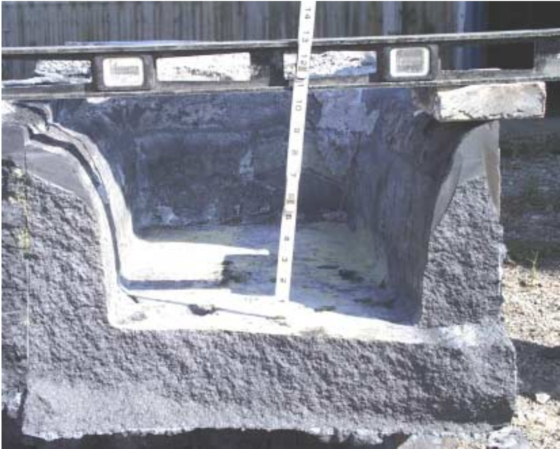
Figure 16 - Cross-section of End Sump Showing Wall Erosion
