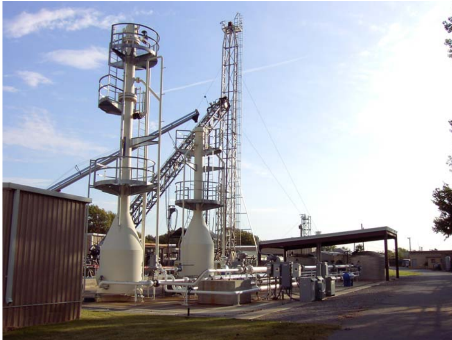
Figure 3.1 ACTS Flow Loop with Separation Tower and Cuttings Injection Hopper with Loading Auger
