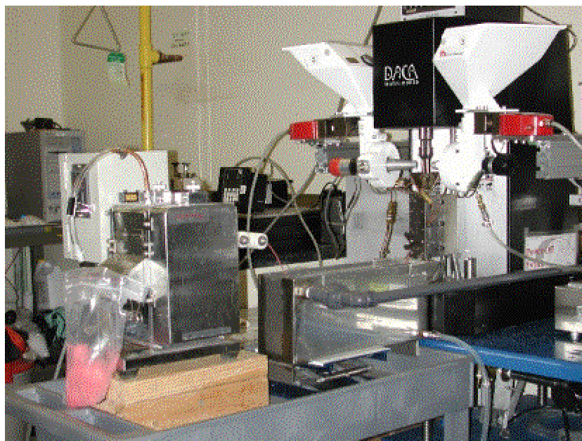
Figure 47. Microcompounder with two loss-in-weight feeders, water bath, and pelletizer.
