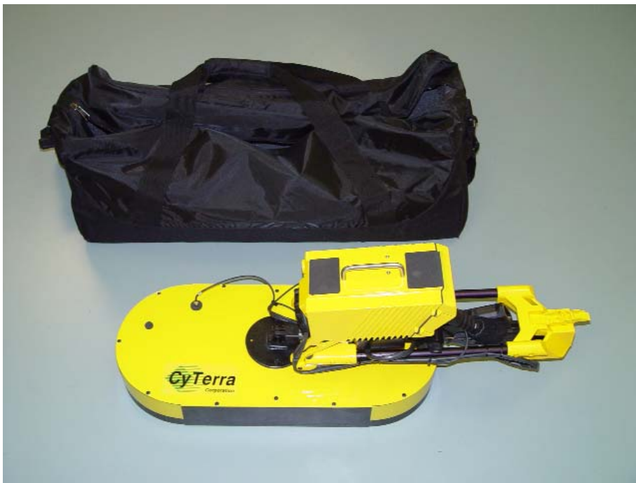
Figure 2.2-2. The compact, lightweight, foldout handheld detector is a key improvement.
