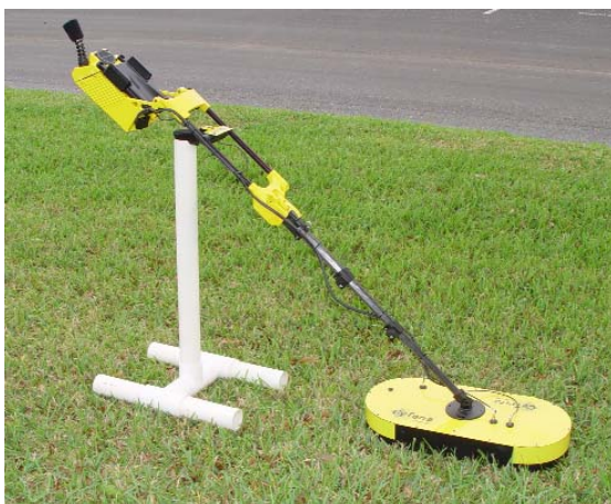
Figure 5.0-1. Successful user friendly buried plastic pipe detection has been demonstrated by CyTerra in local sandbox and backyard locations using LULU
