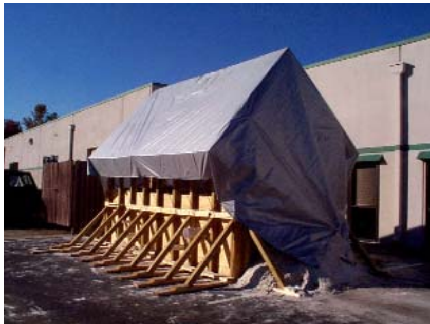
Figure 4.0-1. The sandbox was interlaced with several plastic pipe targets to allow for early hardware and algorithm tests prior to field testing
