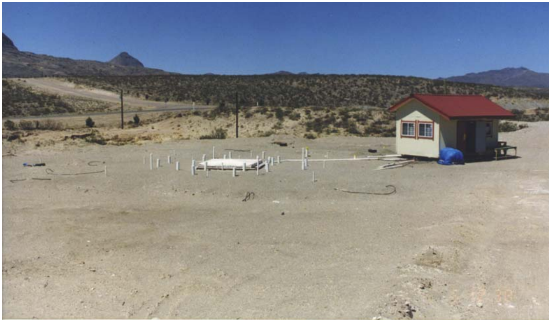
Figure 2: View of the site looking to the northwest. The infiltrometer covered by the white PVC tarp just to the left of center in the photograph. Surrounding the infiltrometer in an axi-symmetric pattern are 13 PVC access tubes (smaller diameter pipes) and covers for the tensiometer access tubes (larger diameter pipes). The building houses all of the data acquisition equipment and water/tracer supply tanks and equipment. The center access tube discussed later in this report is located at the center of the infiltrometer and is covered by the tarp.
