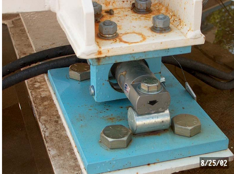
Figure 5.4 – One of Three Load Cells under Injection Tower
