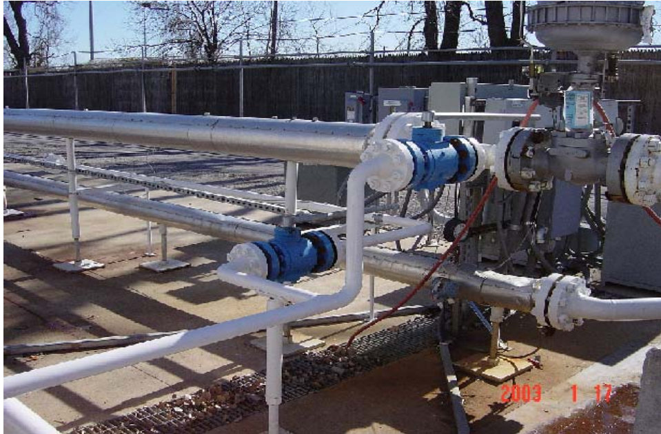
Figure 5.2 - Flushing System for ACTS Flow Loop
