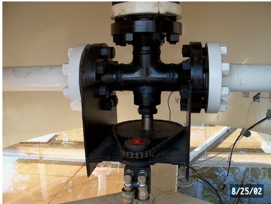
Figure 5.1 – Cuttings Injection into 4-inch Flowline
