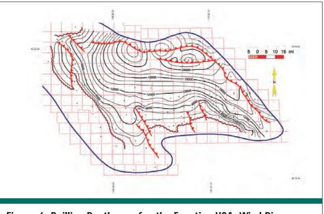
Figure 6: Drilling Depth map for the Frontier UOA, Wind River Basin (Depth is to the mid-point of the UOA)
