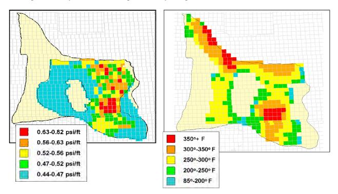
**Figure 14:** *Example maps of engineering parameters: Left – Reservoir pressure gradients per township for the Lower Mesaverde UOA, GGRB. Right - Reservoir temperature for the Frontier UOA, GGRB.*
