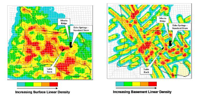
**Figure 17:** Two components in the calculation of structural complexity. Right: Basement component as determined from remote sensing data (magnetic and gravity): Left: Surface component based on density of mapped surface lineaments.
