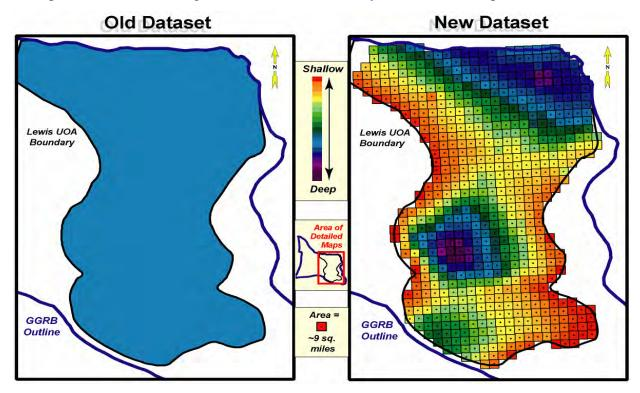
**Figure 23:** Comparison of previously-existing NETL model characterization (left) with dataset prepared in this study (right) with regard to description of drilling depth. Example is from the Lewis UOA, GGRB.
