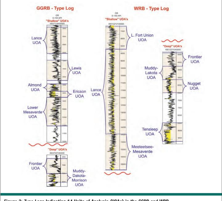
Figure 2: Type Logs Indicating 14 Units of Analysis (UOAs) in the GGRB and WRB
