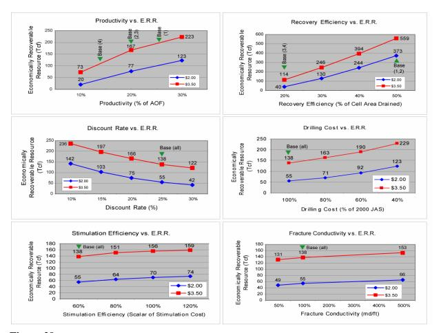
**Figure 29:** Sensitivity of GSAM estimates of economically-recoverable resources to incremental changes in key model parameters that are used to represent technology advance. The green triangles indicate the settings for these values for unique portions of the base case ("1" = marginal marine UOAs, "2" = basinal UOAs, "3" = fluvial UOAs, and "4" = thick fluvial UOAs.
