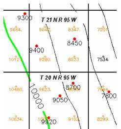
**Figure 21:** An example of a gridded dataset – in this case drilling depths. Red dots are well locations. Orange values mark the centers of grid cells - in this example, cells are 9 mi<sup>2</sup> in size. Each cell is assigned a unique depth based on computer extrapolation of scattered well data.
