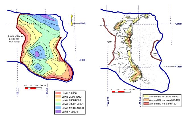
**Figure 11:** *Example Geologic Maps: Left - Drilling depth to mid-point of the Lewis UOA, GGRB, Sandstone isochore map for marginal-marine Almond "B2" sandstones, GGRB. A complete archive of maps and cross-sections created during this study is presented elsewhere on this CD.*
