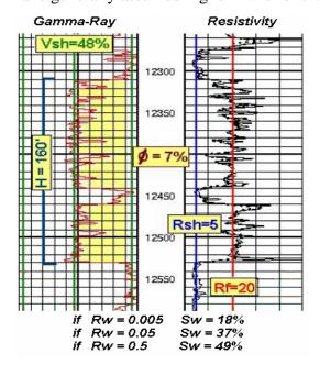
values for marine and near-shore UOAs. We have also generally assumed decreasing Rw with depth. For example, in the Frontier and Dakota UOAs in the GGRB, Rw was set to range from 0.04 for cells with the greatest drilling depths to 0.09 for those with the shallowest drilling depths.
