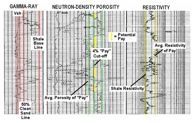
**Figure 12:** Sample well log showing the key elements of the well log analysis procedure. "Potential Pay" is the thickness of interval characterized for each UOA. The average values for Vsh,, Porosity, and Resistivity are all relative to the potential pay intervals only
