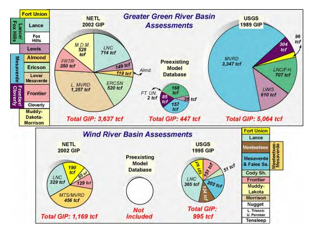
**Figure 25:** Summary of the gas-in-place results of this study ("NETL 2002 GIP") with in-place resource characterizations previously available to NETL's analytical models databases and the findings of previous USGS gas-in-place studies (GGRB, 1989; WRB, 1995). Top: Results for the Greater Green River basin; Bottom: Results for the Wind River basin. Color keys to pies are provided. Pie size is proportional to total in-place resource.
