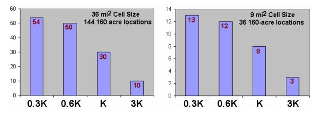
**Figure 22:** *Procedure for distributing a range of permeability within grid cells based on estimated average cell permeability.*
