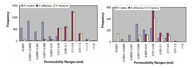
**Figure 27:** Distribution of matrix, natural fracture, and total effective permeability in two representative UOAs. Frequency refers to the number of <sup>1</sup>/<sub>4</sub>-township grid cells. Left – data from the Lewis UOA, GGRB; Right – data for the Meeteetsee-Mesaverde UOA, WRB.
