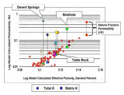
**Figure 19:** *Method for partitioning effective permeability into matrix and natural fracture overprint components. Example from the analysis of the Lewis UOA, GGRB.*
