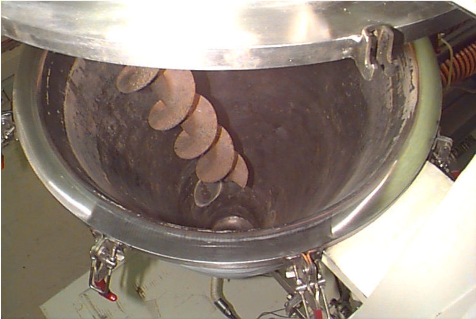
Figure 3. View of inside of Ross vertical cone mixer.
