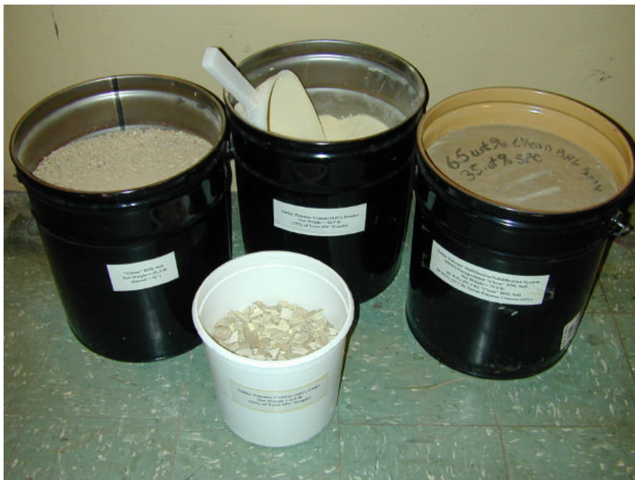
Figure 8. Volumetric Comparison of SPSS Batch Components and Final Waste Form (right).
