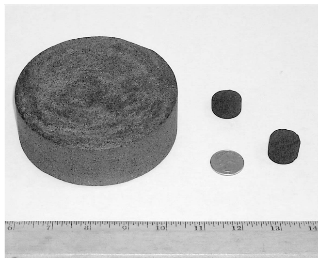
Figure 3. Gas storage monolith and test specimens
