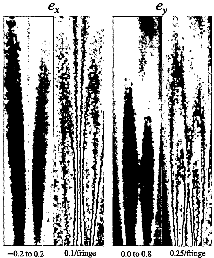
Figure 11. COLOR MAP AND SIMULATED INTERFEROGRAM OF THE COMPONENTS OF THE ECCENTRICITY VECTOR MEASURED WITH 8 \times 8 -PIXEL SUBIMAGES. THE COLOR-MAP RANGES AND FRINGE SPACINGS ARE INDICATED BENEATH THE IMAGE IN UNITS OF PIXELS/IMAGE DELAY.
