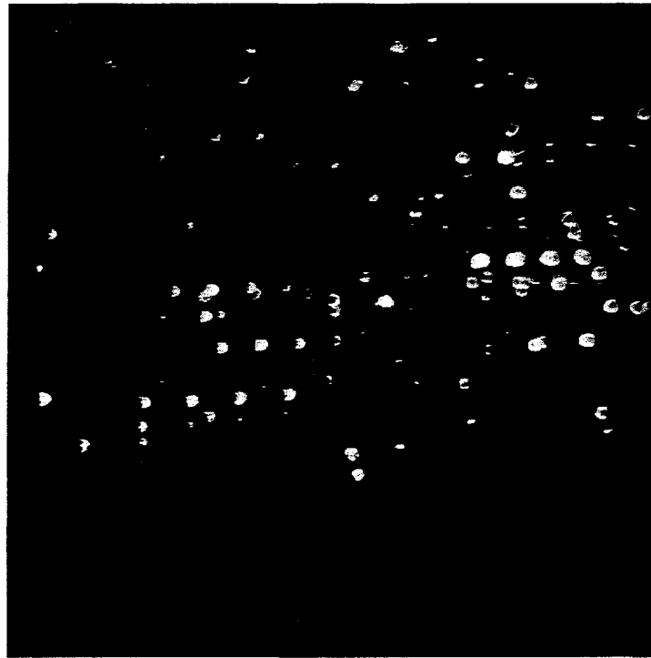
Figure 32. Particles imaging for rectangular nozzle at P =82 psi (nozzle orientation, see Figure 27).
