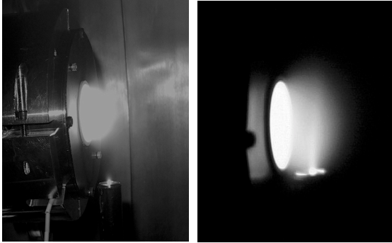
Fig. 10 Cylindrical thruster in stable (a) and unstable (b) operating regimes. The plume is visually more diffused in the unstable regime.
