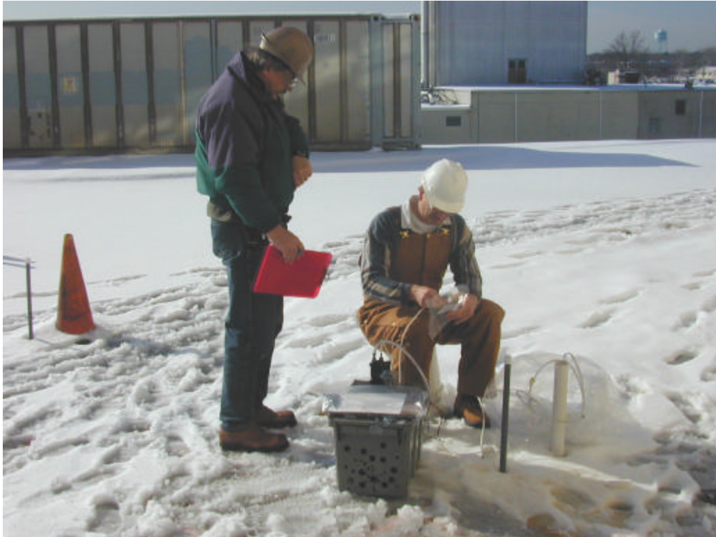
Figure 13. Collecting air samples from an external port
