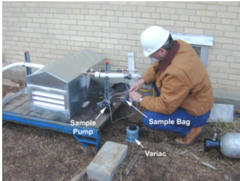
Figure 10. Air sample being collected at the south circulation loop
