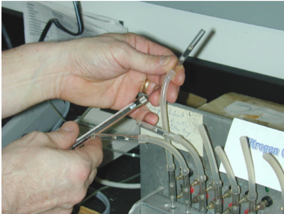
Figure 14. Injection of sample onto a Capillary Adsorbent Tracer Sampler (CATS)
