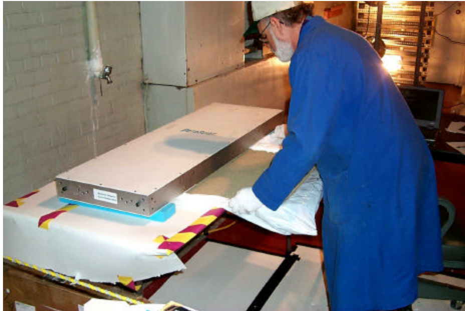
Figure 1. Illustration of BetaScint™ Spectrometer and Soil Sample in Tray
