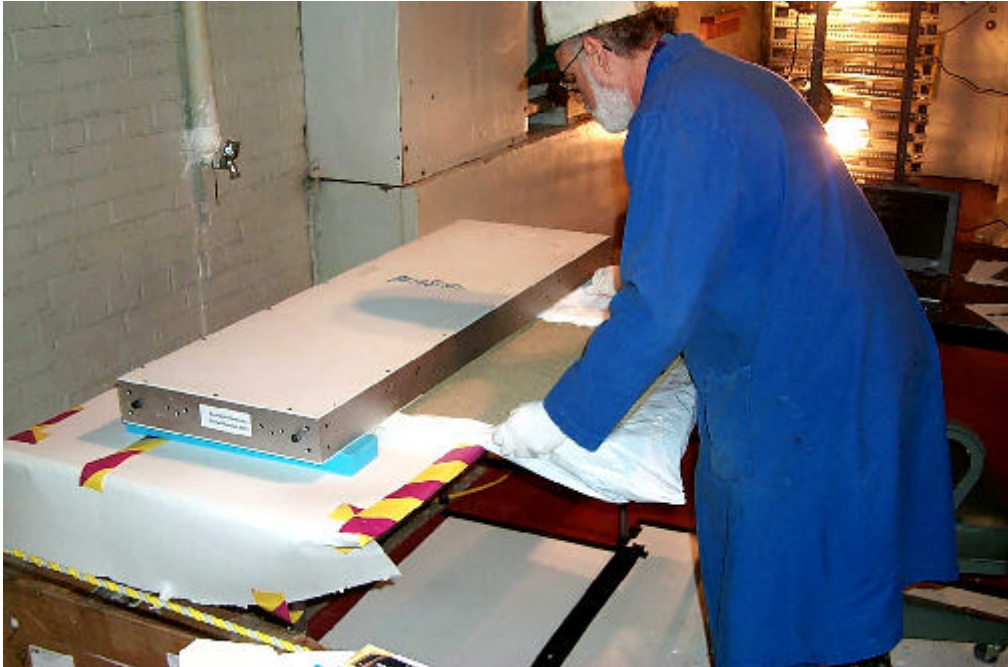
Figure 4 Loading soil sample for Sr-90 BetaScint analysis at BNL
