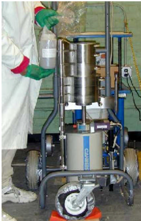
Figure 4-7. ISOCS instrument configured for sample analysis
