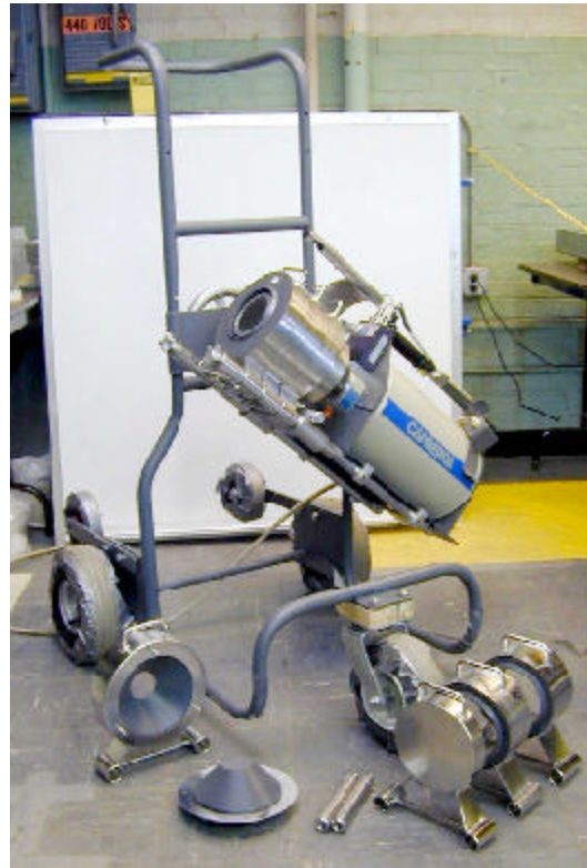
Figure 2-2. ISOCS cart with detector, cryostat and modular shield system
