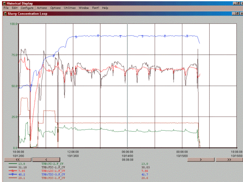
Fig. 39. Slurry concentration loop operation during Batch 2 (45°C) of Test 4. (Blue—Temperature, 0–50°C; Brown and green—pre- and post-filter pressure, 0–100 psi; Black—Filtrate flow, 0–50 mL/min; Red—Tank level, 0–11 in.)
