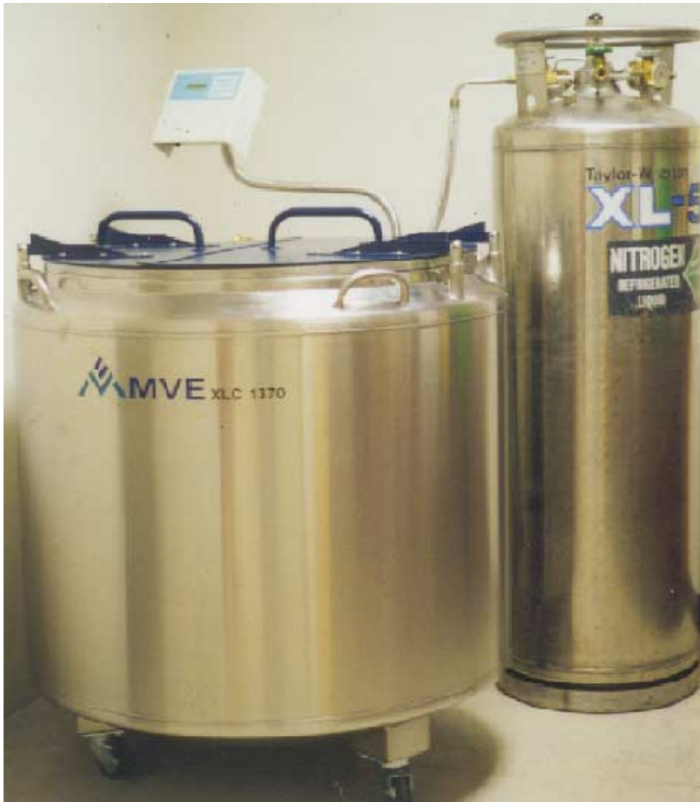
Figure 5. Example of a liquid nitrogen tank where chinook salmon and steelhead germplasm is stored.
