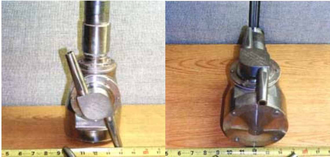
Figure 3.4 Wash ball showing the dual opposed nozzles.
