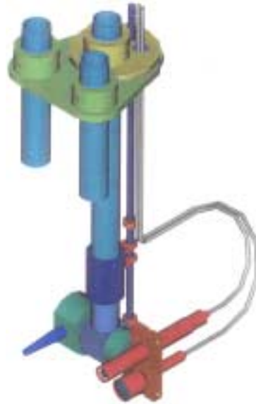
Figure 3.5 Directional nozzle, light, and camera configuration
