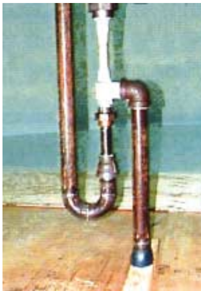
Figure 3.7 Model of steam jet used during retrieval tests
