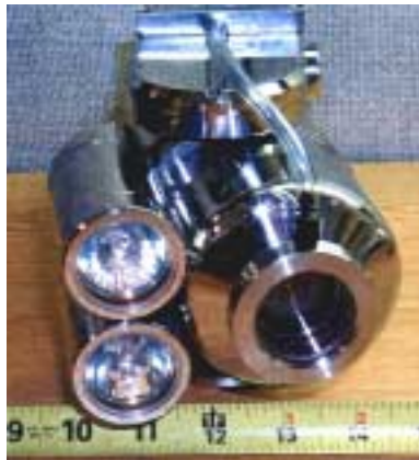
Figure 3.6 Video camera showing lights and purge air ring
