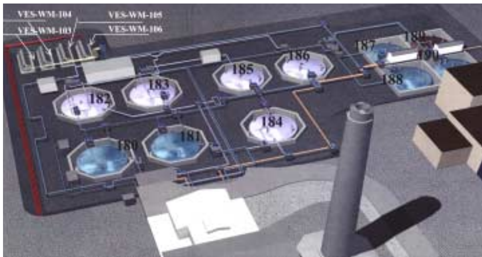
Figure 3.1 INTEC tank farm overview showing the 1136-m 3 (300,000-gal.) tanks and vault types
