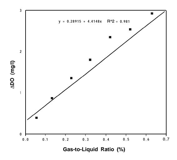
Figure 12 The Change in Dissolved Oxygen (ADO) as a Function of Gas-to-Liquid Ratio - 30 Inch Column
