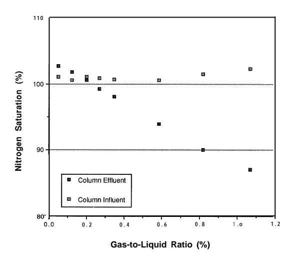
Figure 8 Influent and Effluent Nitrogen Saturation as a Function of Gas-to-Liquid Ratio - 24 Inch Column
