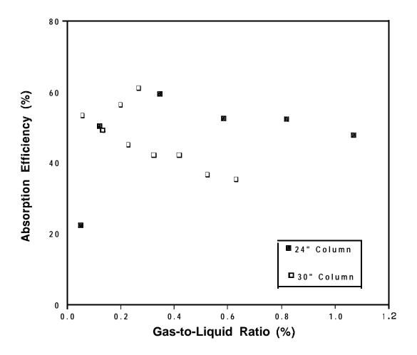
Figure 23 Absorption Efficiency as a Function of Gas-to-Liquid Ratio and Column Size
