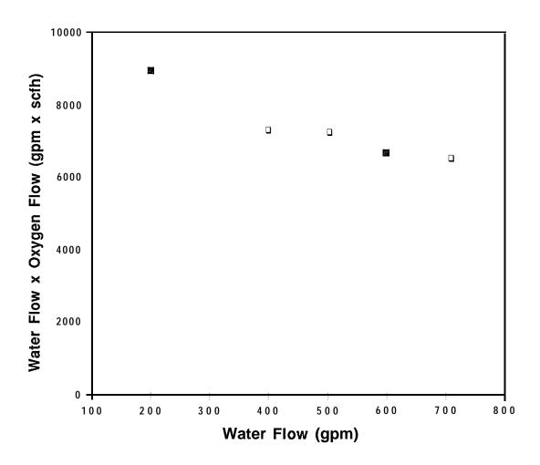
Figure 10 The Product of Water Flow x Gas Flow as a Function of Water Flow in Test 2 - 24 Inch Column
