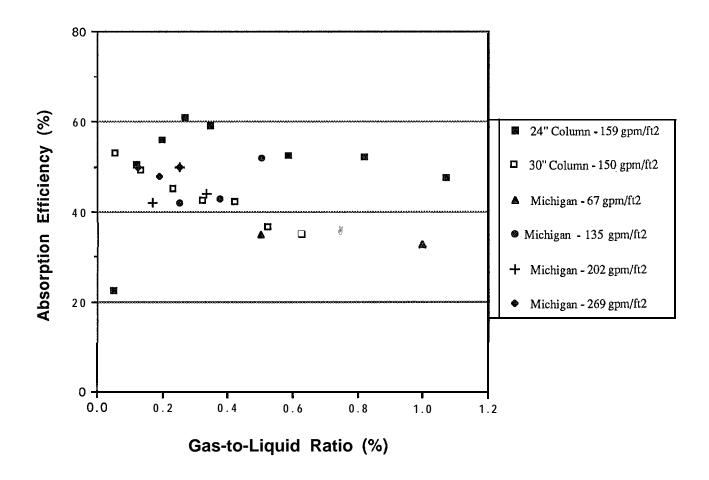
Figure 24 Comparison of Absorption Efficiency at Williamette Hatchery with Michigan Pure Oxygen Columns (Westers et al, In Press)
