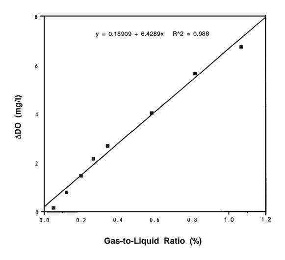
Figure 3 The Change in  ${\tt Dissolved}$  Oxygen (ADO) as a Function of Gas-to-Liquid Ratio - 24 Inch Column
