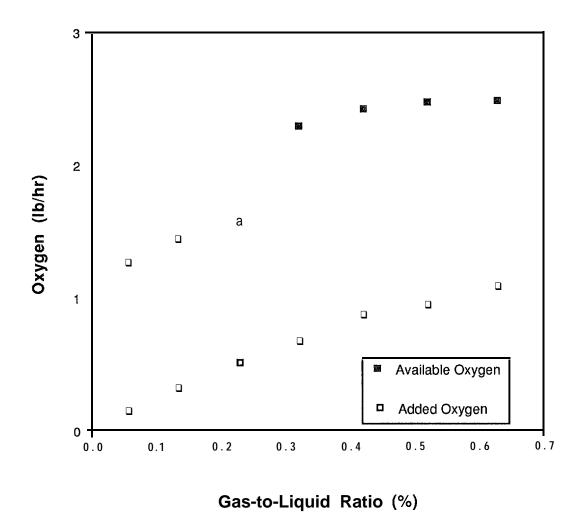
Figure 15 Oxygen Transfer Rate and Available Oxygen (based on an effluent criteria of 7 mg/l) as a Function of Gas-to-Liquid Ratio - 30 Inch Column
