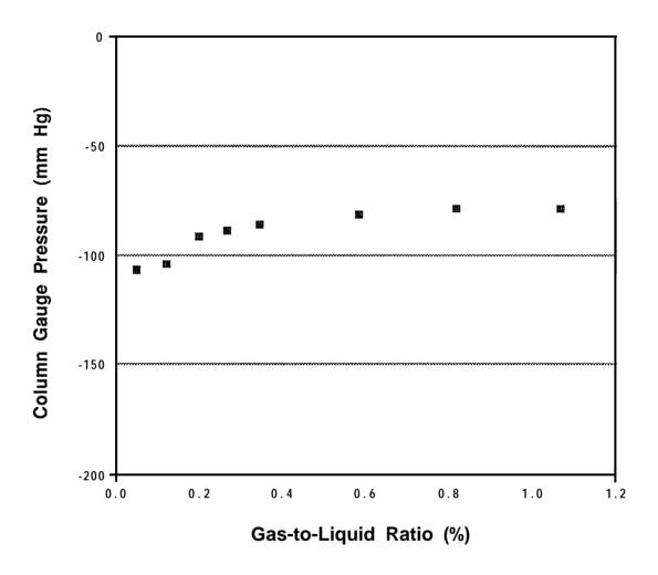
Figure 9 Gauge Pressure on Top of Column as a Function of Gas-to-Liquid Ratio - 24 Inch Column
