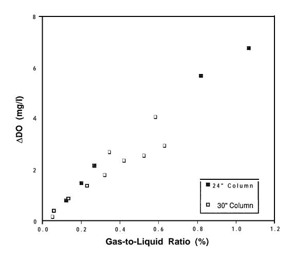
Figure 21 The Change in Dissolved Oxygen (ADO) as a Function of Gas-to-Liquid Ratio and Column Size
