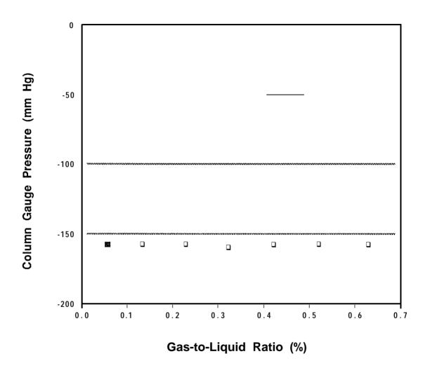
Figure 18 Gauge Pressure on Top of Column as a Function of Gas-to-Liquid Ratio - 30 Inch Column
