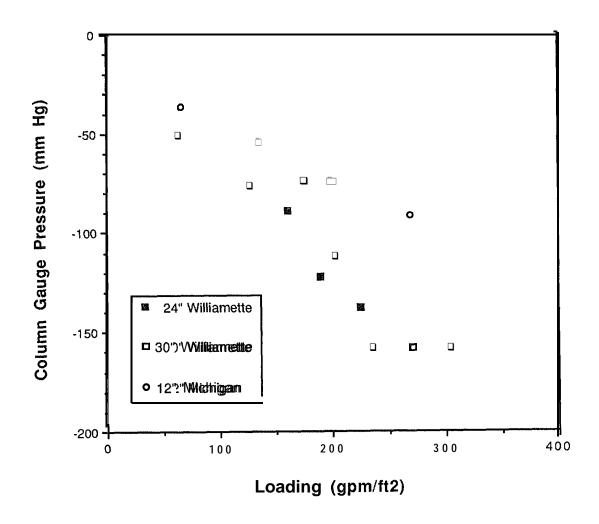
Figure 25 Effect of Hydraulic Loading on Column Pressure (based on Westers et al., In Press and the 24 inch column at Williamette)
