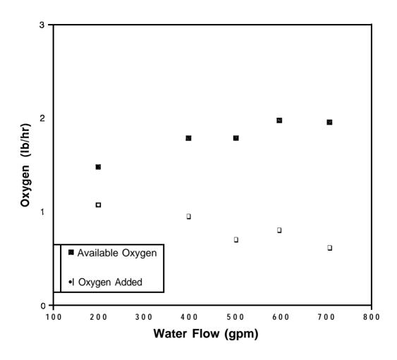
Figure 11 Oxygen Transfer Rate and Available Oxygen (based on an effluent criteria of 7 mg/l) as a Function of Water Flow Rate in Test 2 - 24 Inch Column
