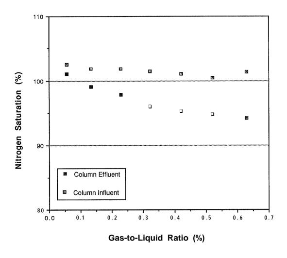
Figure 17 Influent and Effluent Nitrogen Saturation as a Function of Gas-to-Liquid Ratio - 30 Inch Column
