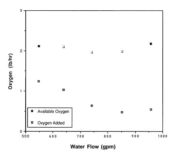
Figure 20 Oxygen Transfer Rate and Available Oxygen (based on an effluent criteria of 7 mg/l) as a Function of Water Flow Rate in Test 4 - 30 Inch Column
