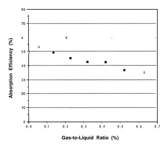
Figure 13 Absorption Efficiency as a Function of Gas-to-Liquid Ratio - 30 Inch Column
