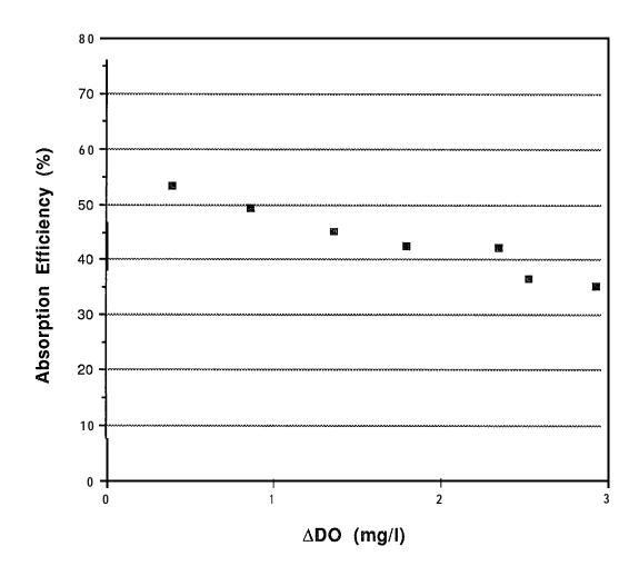
Figure 14 Absorption Efficiency as a Function of ADO - 30 Inch Column
