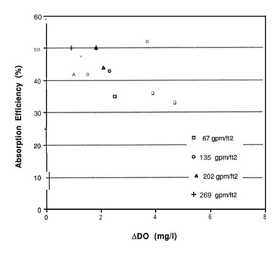
Figure B-3 Absorption Efficiency as a Function of **ADO** and Hydraulic Loading Rate - 12 Inch Column (Westers et al., In Press)
