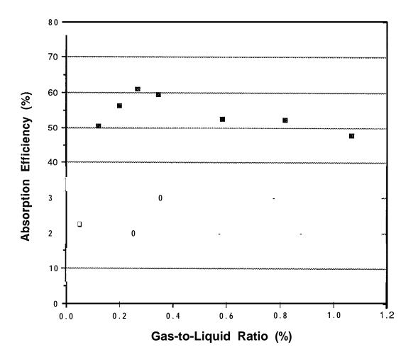
Figure 4 Absorption Efficiency as a Function of Gas-to-Liquid Ratio - 24 Inch Column
