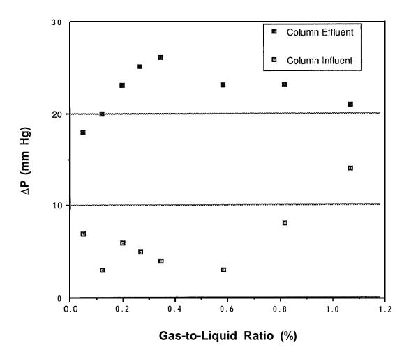
Figure 7 Influent and Effluent AP as a Function of Gas-to-Liquid Ratio - 24 Inch Column
