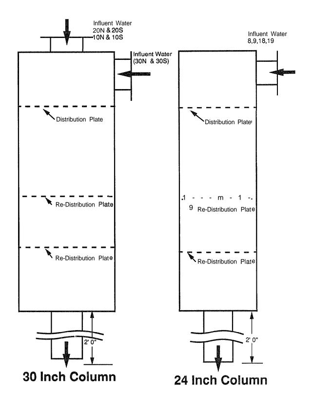
Figure 1 Diagram of 24 and 30 Inch in Diameter *Williamette Hatchery Oxygen Transfer Columns.*
