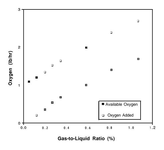
Figure 6 Oxygen Transfer Rate and Available Oxygen (based on an effluent criteria of 7 mg/l) as a Function of Gas-to-Liquid Ratio - 24 Inch Column
