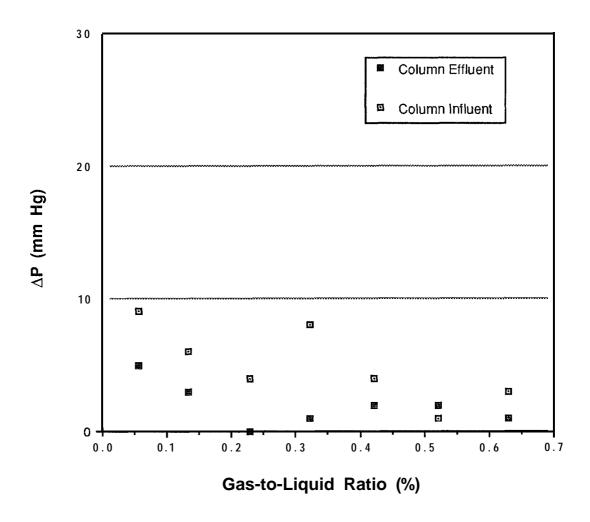
Figure 16 Influent and Effluent AP as a Function of Gas-to-Liquid Ratio - 30 Inch Column
