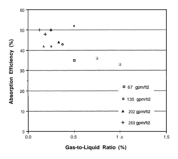
Figure B-2 Absorption Efficiency as a Function of Gas-to-Liquid Ratio and Hydraulic Loading Rate - 12 Inch Column (Westers et al., In Press)
