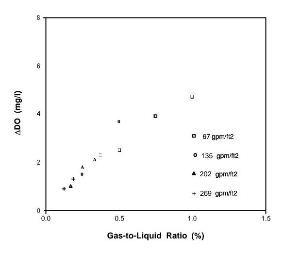
Figure B-I The Change in Dissolved Oxygen (ADO) as a Function of Gas-to-Liquid Ratio and Hydraulic Loading Rate - 12 Inch Column (Westers et al., In Press)
