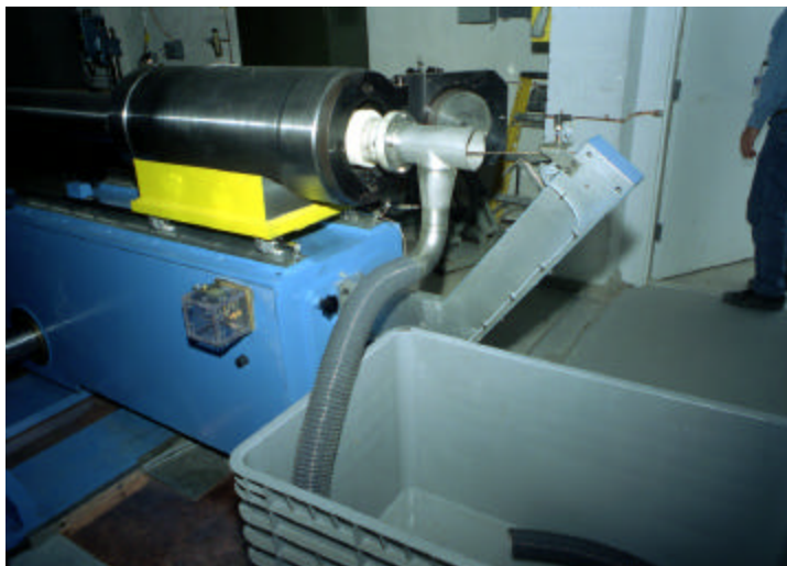
Figure 2a: Pump Tube-Cleaning Machine at Breech
