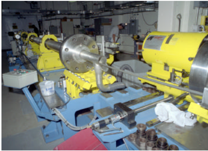
Figure 2b: Pump Tube Cleaning Machine at Acceleration Reservoir
