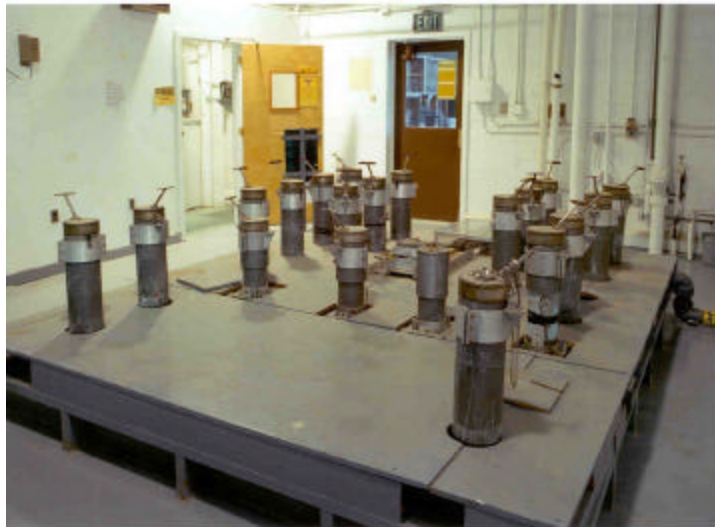
Figure 1 View of the GIF room in 1994, with shielded air tubes and cover in place.
