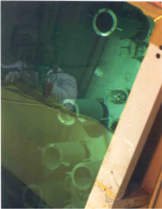
Figure 7 A view of the empty lead casks. Some sources remain in the center rack.
