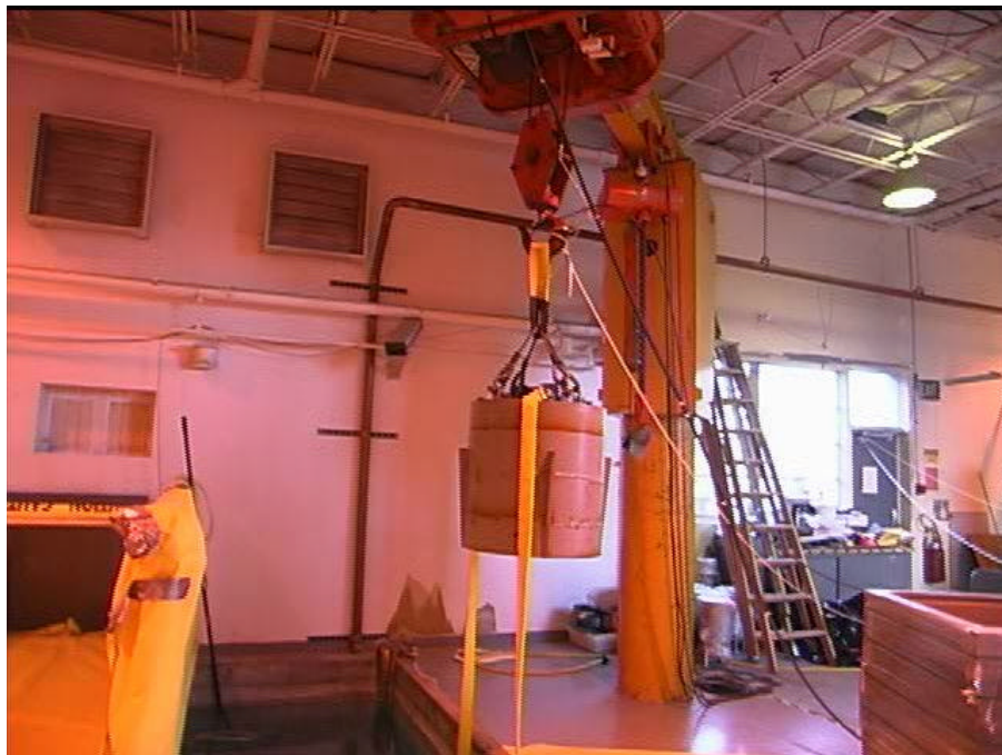
Figure 14 Lifting liner from pool. (Rigging straps were placed remotely while liner was underwater.)
