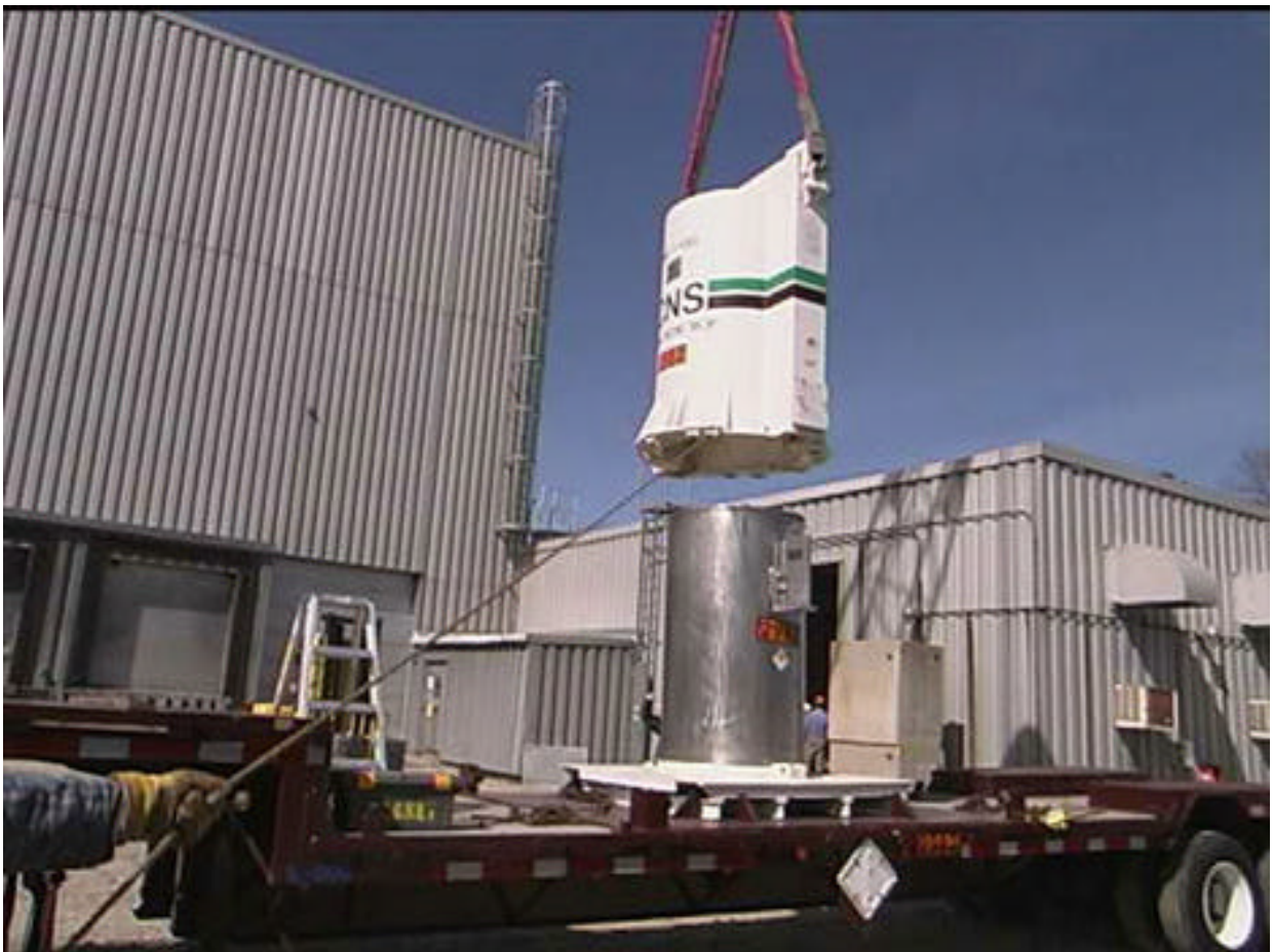
Figure 12 Shipping cask preparation – Removing the impact cover.
