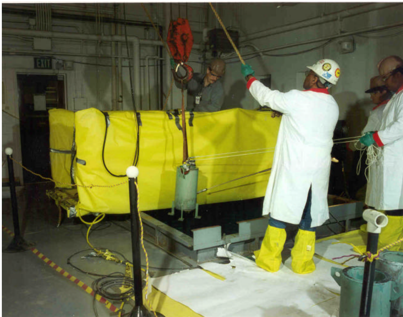
Figure 8 Operator removes lead cask from the pool.
