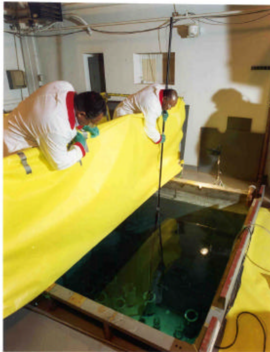
Figure 6 Operators used remote manipulators to move ^{60}\text{Co} Sources from racks to basket.
