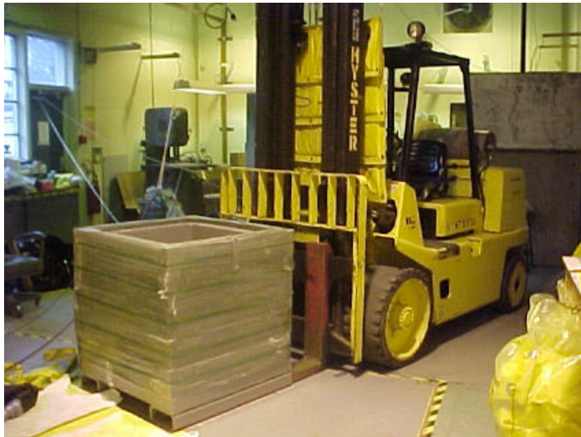
Figure 16 Forklift with shielded transfer box in position next to pool. (Shield wall for crane operator is visible in background to right. The roll-up door was closed for this photo.)
