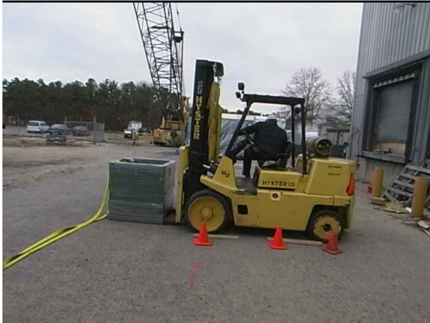
Figure 17 Loaded forklift in parked position outside. (Operator is leaving to go behind shield wall next to Grove crane. Note rigging straps attached to liner in shield box.)
