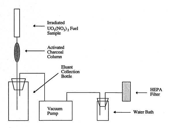
fig.1 Charcoal Filtration Apparatus
