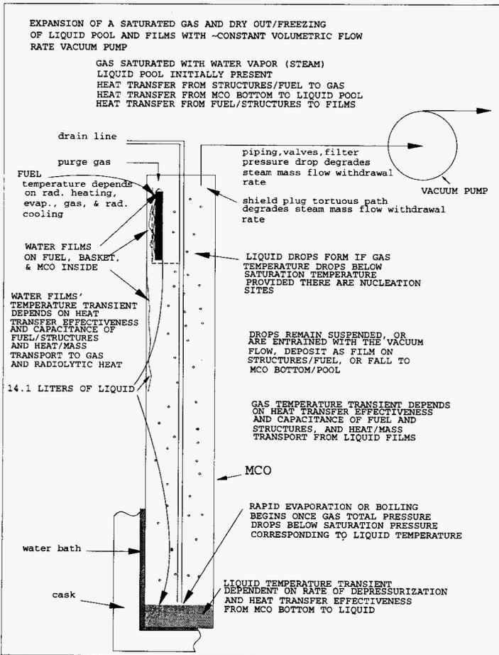
Figure 5.2 Dry Out of Pool and Liq. Films with Const. Vol. Flow Vac. Pump, and Heat/Mass Trans. Between Gas and Liquid and Between Gas/Liquid Phases and Fuel/Structures
