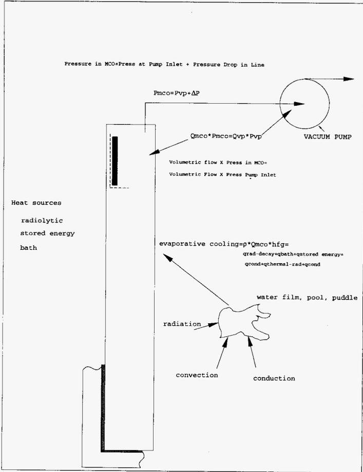
Figure 5.4 Dry Out of Pool and Liq. Films with Const. Vol. Flow Vac. Pump, and Heat/Mass Trans. Between Gas and Liquid and Between Gas/Liquid Phases and Fuel/Structures
