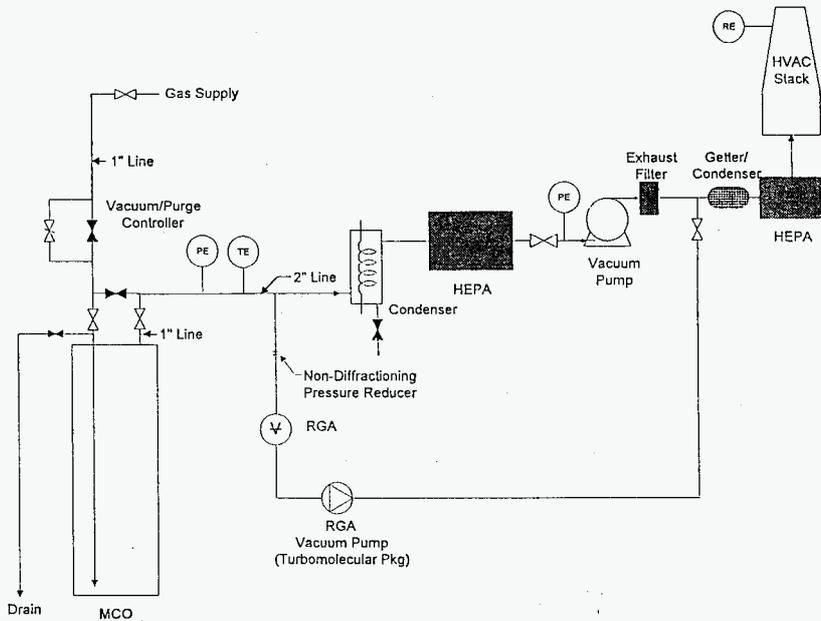
Figure 5.1 Preliminary Schematic of SNF Vacuum System.
