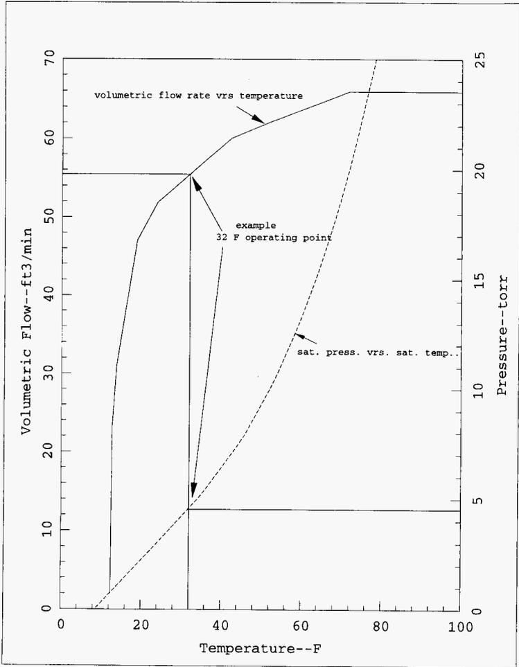
Figure 5.6 SV100 Vacuum Pump--Saturated Steam Pumping Characteristics
