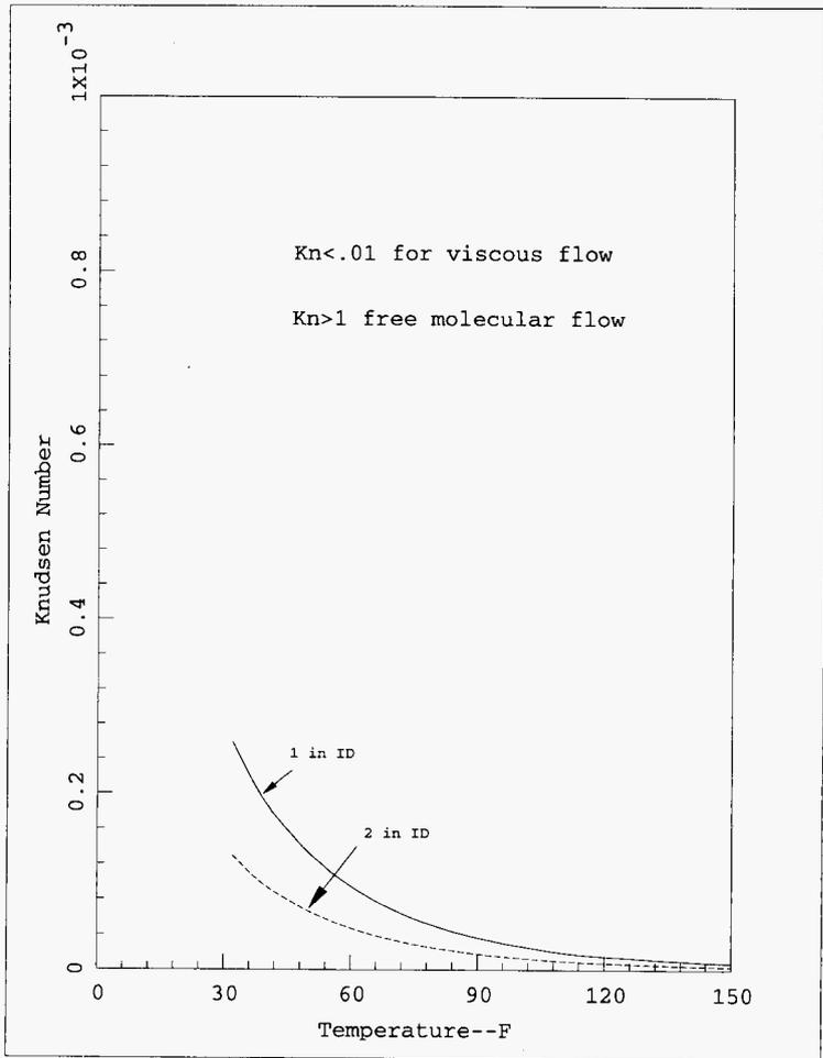
Figure 5.10 Knudsen Number versus Temperature
