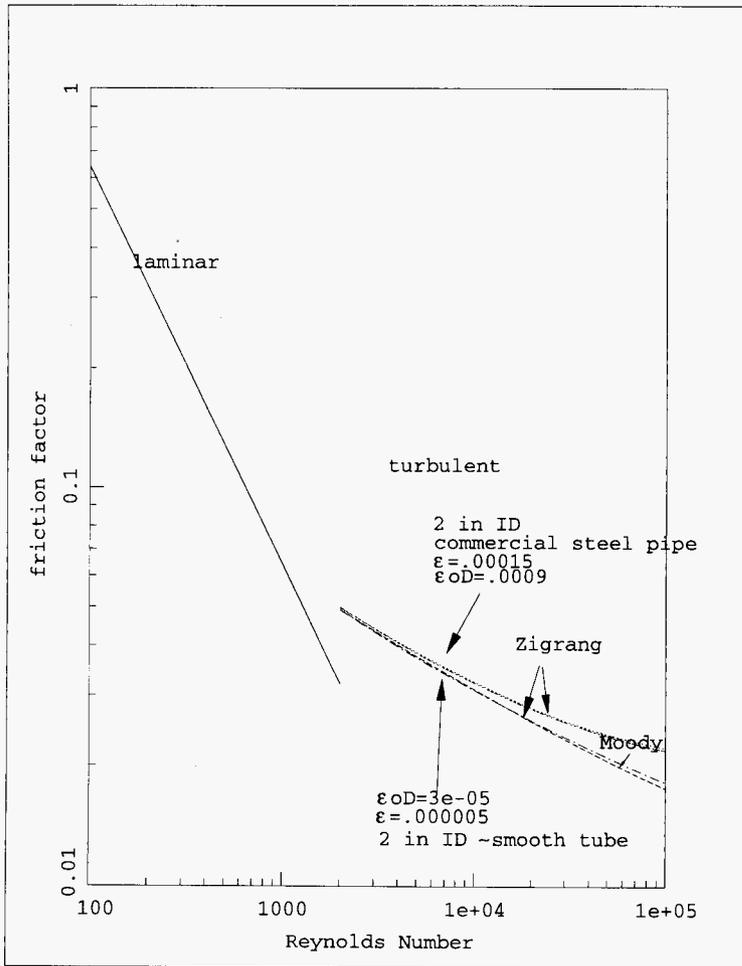
Figure 5.14 Friction factor versus Reynolds Number
