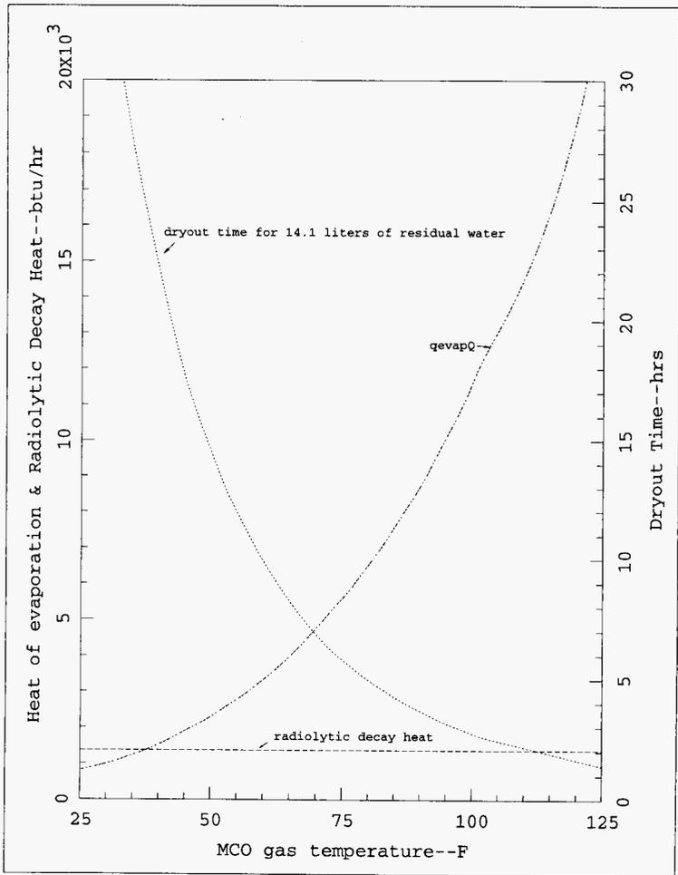
Figure 5.7 Evaporative Heat removal from liquid versus gas temperature, Radiolytic Heat Rate, and Dryout Time
