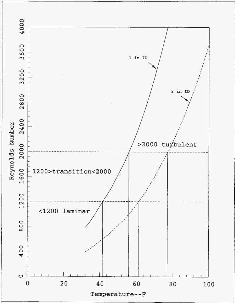
Figure 5.12 Reynolds Number versus Temperature and Laminar/Turbulent Boundaries
