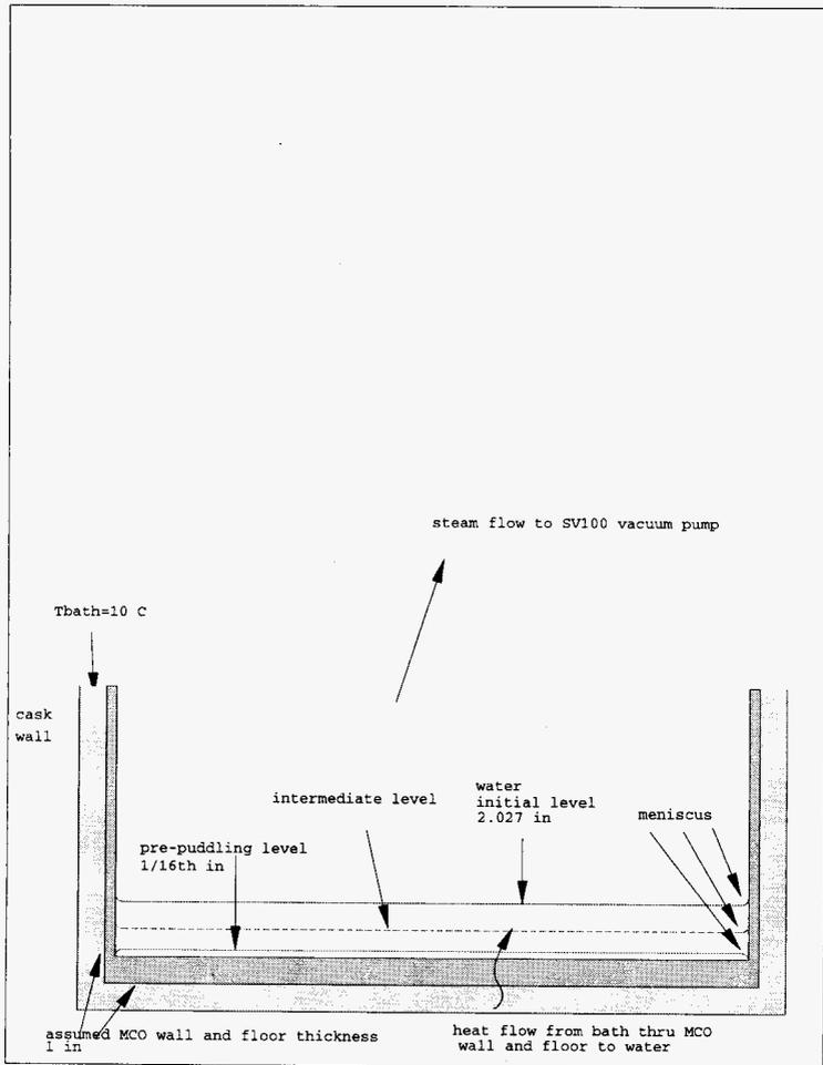
Figure 5.22 Quasi-steady Evaporation of Water Due to Wall Dryout but preceding End Plate Dryout and Puddling
