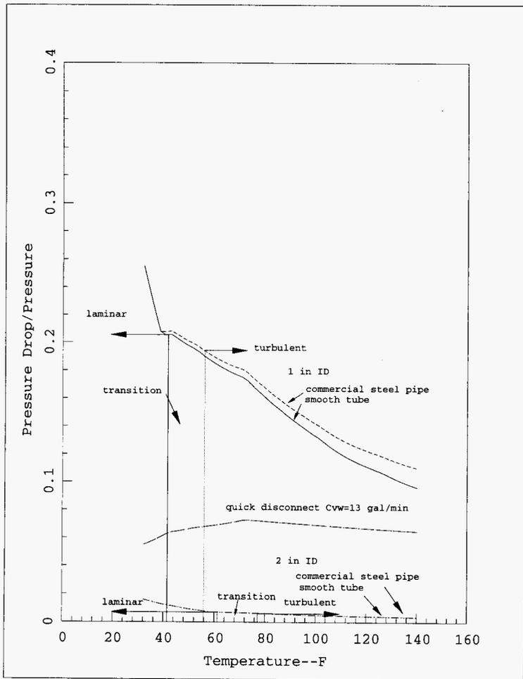
Figure 5.17 Ratio of Pressure Drop/Pressure versus Temperature
