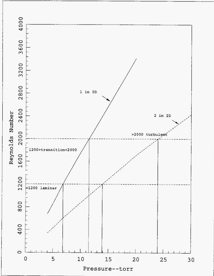
Figure 5.13 Reynolds Number versus Pressure, ID and laminar/turbulent boundaries
