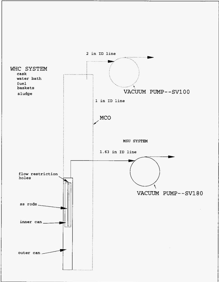
Figure 4.1 WHC & MSU Test Vacuum System & Materials Comparison
