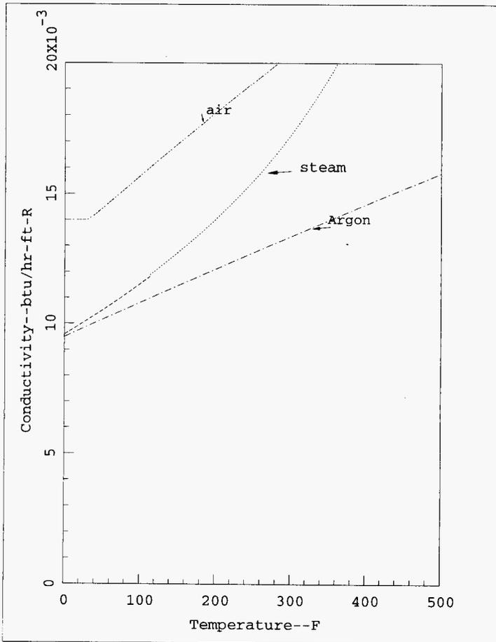
Figure 5.11 Thermal Conductivity of air, Argon, steam versus Temperature
