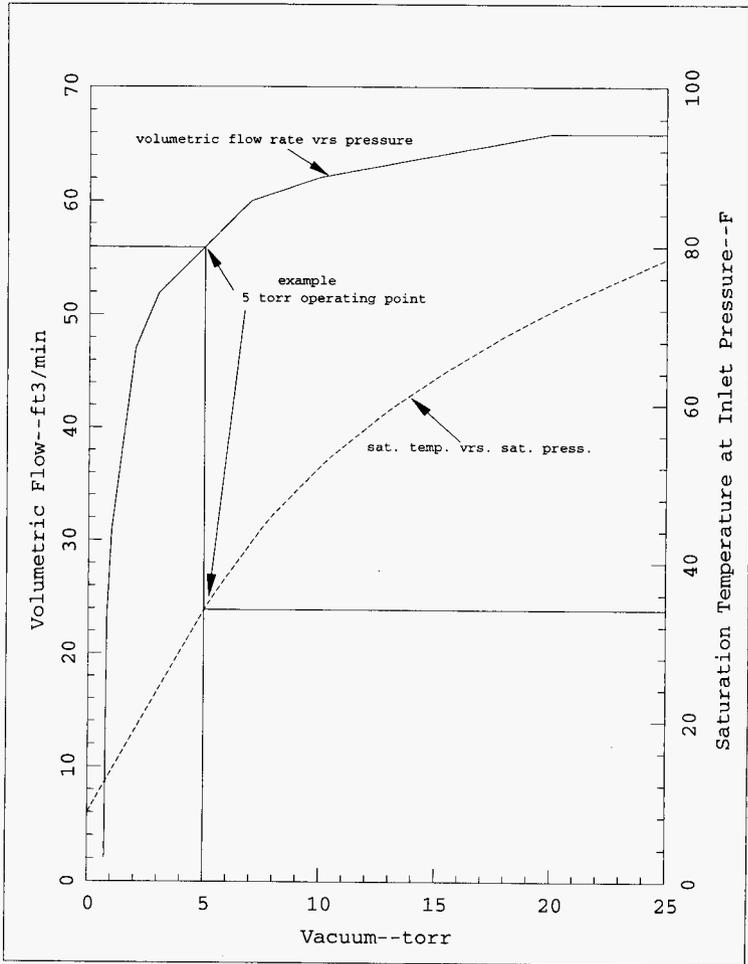
Figure 5.5 SV100 Vacuum Pump--Saturated Steam Pumping Characteristics
