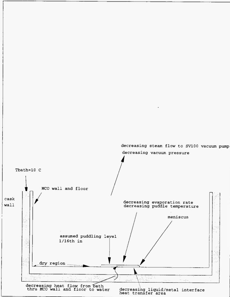
Figure 5.23 Rapid Change in Press., Temp. Liquid/Metal Interface Heat Transfer Area, and Evaporation Rate Caused by Floor Puddling and Dryout Which Could Lead to Freezing
