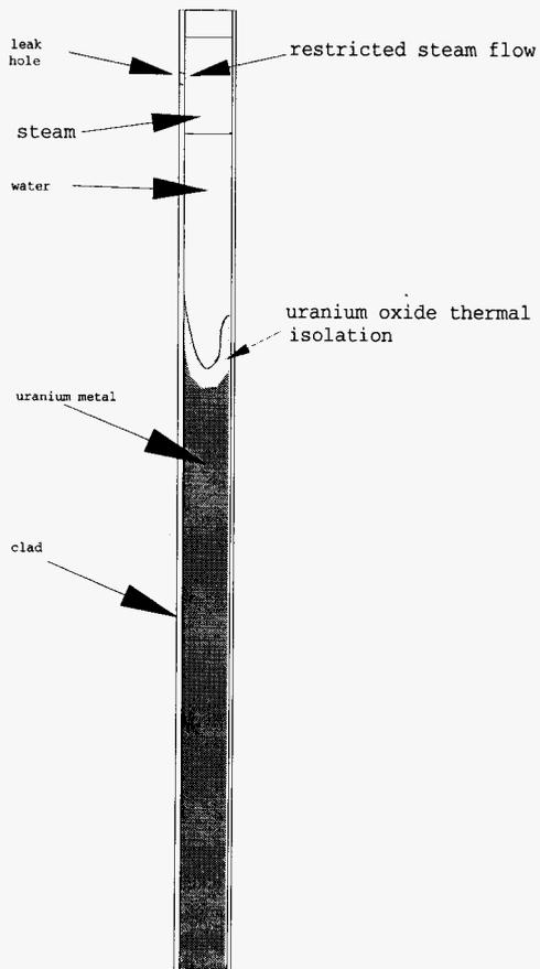
Figure 5.26 Mark-IA Fuel Element Cross Section Showing Possible Residual Water Resulting from Leak Holes and Fuel Wastage Due to Corrosion
