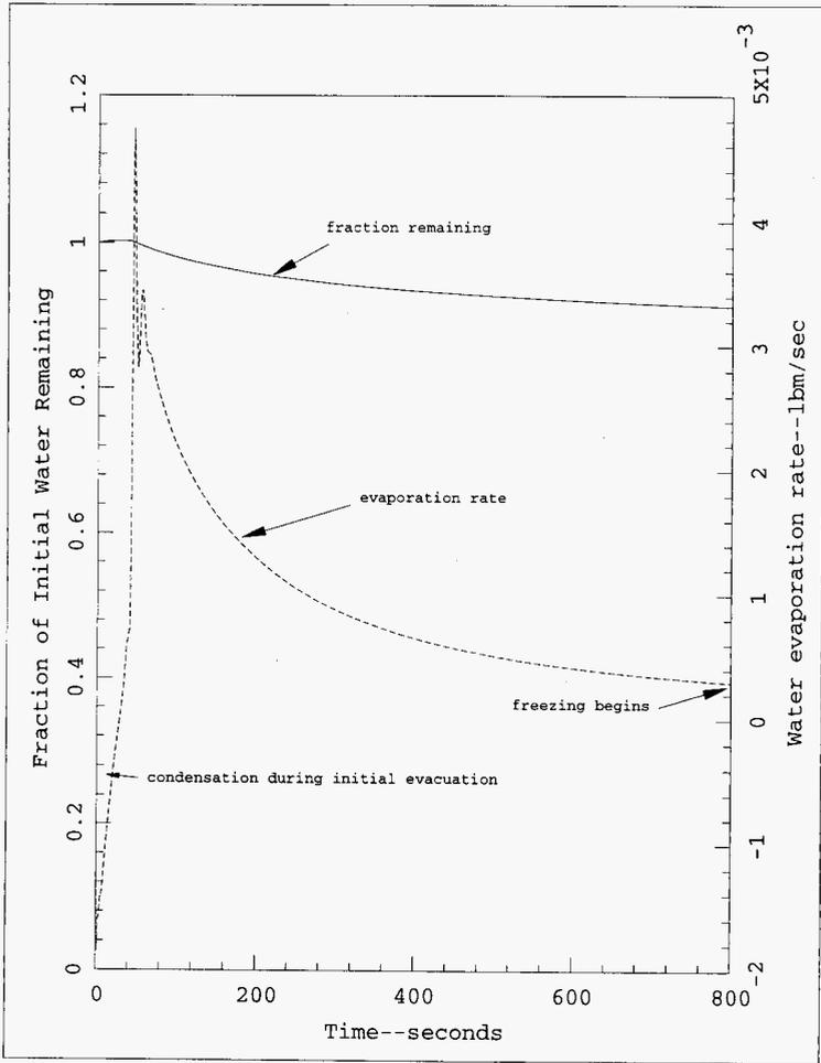
Figure 5.21 Fraction of Initial 4 Liter Quantity of Water Remaining versus Time
