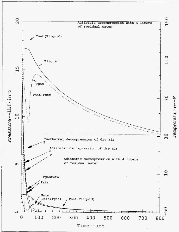
Figure 5.20 Temperature and Pressure Versus Time at a Constant Volumetric Withdrawal rate of 1 ft<sup>3</sup>/sec
