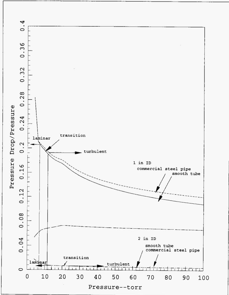
Figure 5.18 Ratio of Pressure Drop/Pressure versus Pressure
