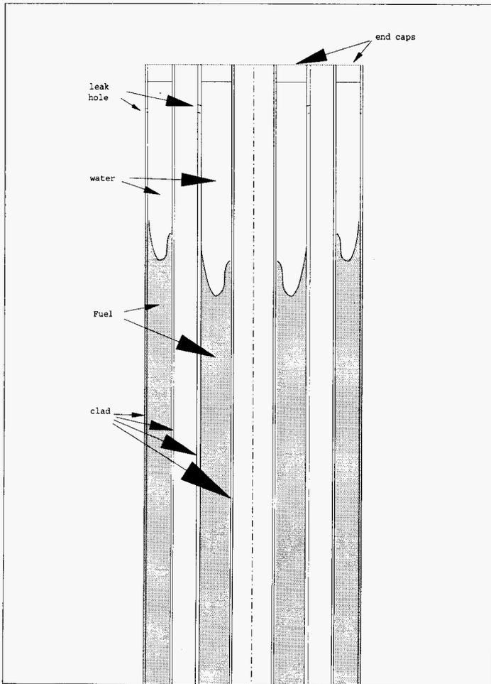
Figure 5.25 Mark-IA Fuel Element Cross Section Showing Possible Residual Water Resulting from Leak Holes and Fuel Wastage Due to Corrosion
