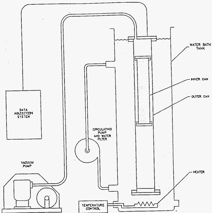
Figure 3.1 MSU Vacuum Drying System Description
