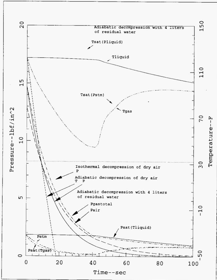
Figure 5.19 Temperature and Pressure Versus Time at a Pump Constant Volumetric Withdrawal rate of 1 ft<sup>3</sup>/sec
