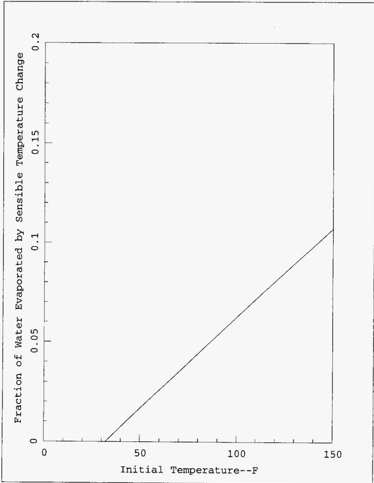
Figure 5.9 Fraction of Water that Can be Evaporated by Sensible Temperature Change of the Water From an Initial Temperature to Freezing
