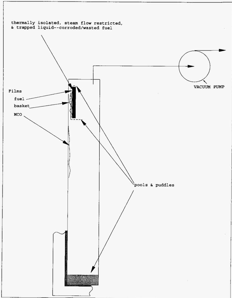
Figure 5.3 Dry Out of Pool and Liq. Films with Const. Vol. Flow Vac. Pump, and Heat/Mass Trans. Between Gas and Liquid and Between Gas/Liquid Phases and Fuel/Structures
