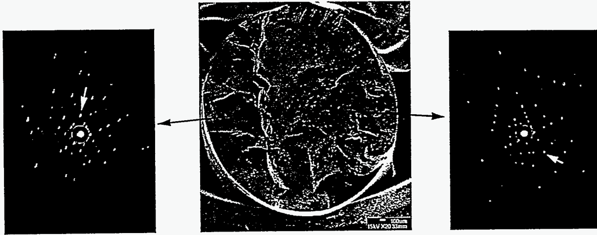
Fig. 5. Fracture surface of a \text{MoSi}_2 bicrystal with a 60^\circ twist boundary about [110] . The arrows in the Laue patterns show crystallographically equivalent poles in both grains. The pole towards the center of the pattern at the intersection of two major zone axes is parallel to \langle 111 \rangle .
