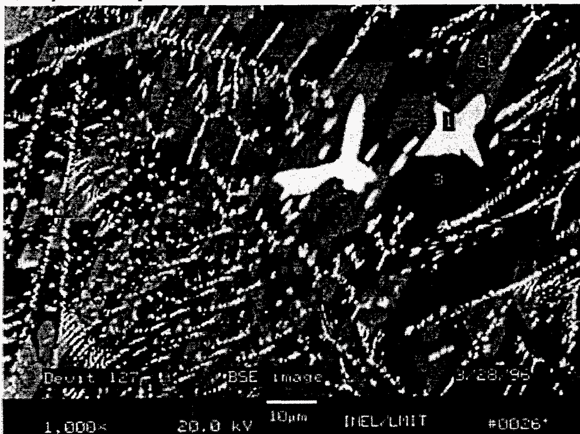
Figure 1: Scanning electron micrograph of an early sample of devitrified Frit 127-based glass containing cerium as a surrogate for plutonium. Brighter areas represent regions of higher average atomic number in this backscattered electron image. The area labeled 1 is the ceria-zirconia-samarium phase, 2 is primarily a calcium silicate phase also containing some zirconium, the bright area labeled 3 is the glassy matrix, and 4 is the sodium calcium aluminosilicate phase.
