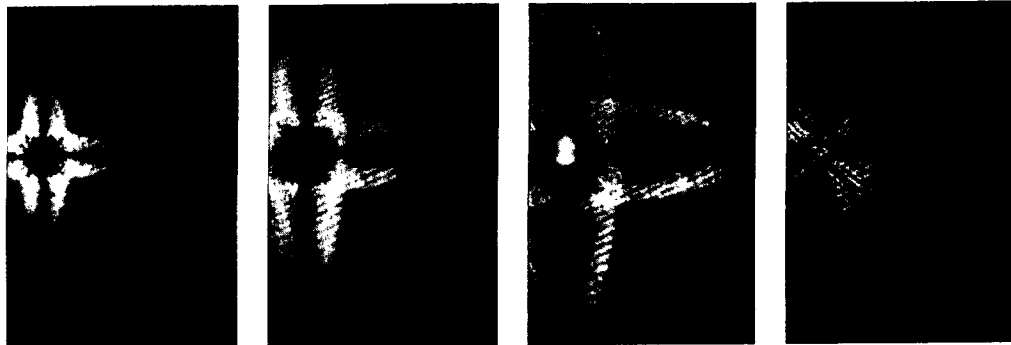
Fig. 3. Time-resolved images during laser-induced damage with higher absorbed laser fluence than in the event shown in Fig. 2. From left to right the images are taken at 20 ns, 40 ns, 60 ns, and 2 s time delay. Images taken through crossed-polarizers and 355 \mu\text{m} in horizontal dimension.
