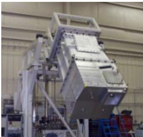
Figure 4. A full-scale Final Optics Assembly was built for testing at LLNL (left). A technician demonstrates the clean and efficient changing of a debris shield.
