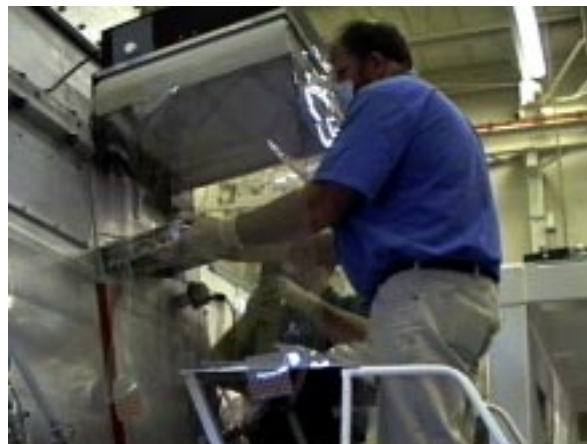
Figure 4. A full-scale Final Optics Assembly was built for testing at LLNL (left). A technician demonstrates the clean and efficient changing of a debris shield.
