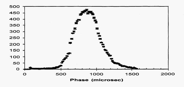
Figure 2. UCN production rate vs rotor phase with respect to the proton pulse on target.
