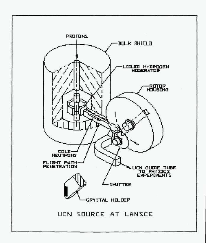
Figure 1. Schematic view of the UCN rotor source at the MLNSC
