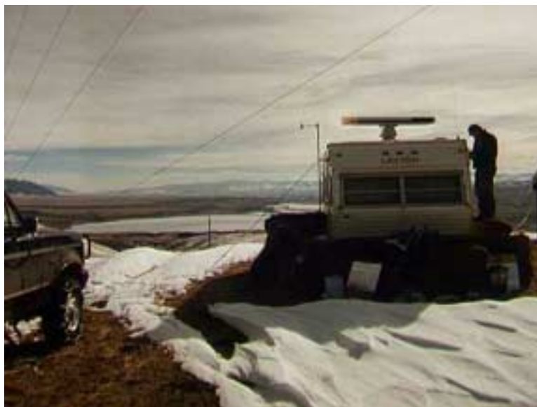
Figure 2. Radar monitoring station, Norris Hill Wind Resource Area, Madison County, Montana. View is toward south. Scanning radar antenna is on trailer roof.
