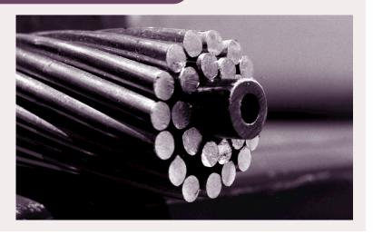
The new composite-reinforced aluminum conductor is stronger, lighter, and has a higher current capacity than conventional utility transmission lines.
