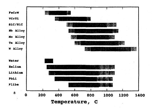
Fig. 5 Estimated operating temperature ranges for candidate structures and coolants
