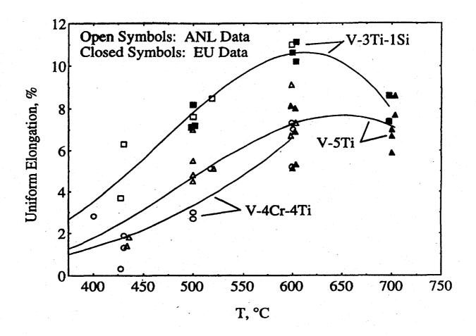
Fig. 2 Uniform elongation of irradiated (6-33 dpa) vanadium alloys compared to irradiated (~ 36 dpa) F82H (test temperature ≈ irradiation temperature).
