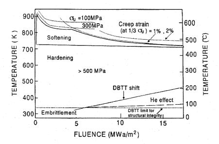
Fig. 4 Schematic design window for a tokamak-type fusion reactor with a ferritic steel first-wall structure (Hishinuma et al.)
