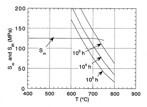
Fig. 3 Primary tensile and creep stress design limits as a function of temperature and time for a vanadium alloy structure
