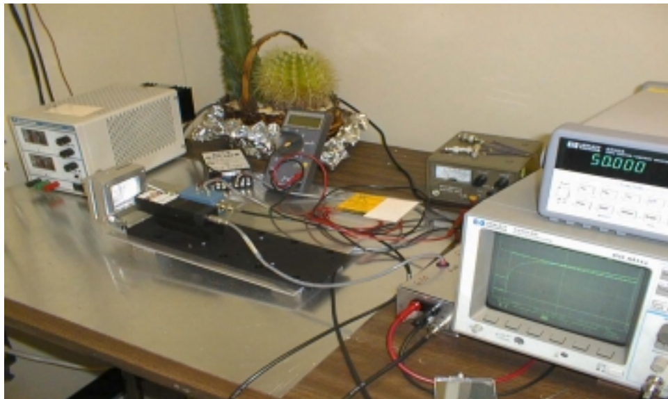
Figure 20. Photograph of the PVCD bench-test system. The oscilloscope is displaying the waveforms of the laser pulse (the step function) and the output of the PVCD. Notice the similarity between the stored traces on the oscilloscope and the waveforms in Figure 18.
