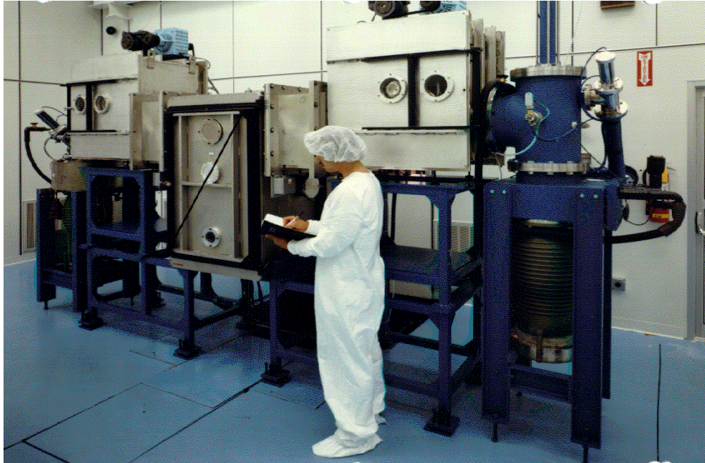
Figure 27. United Solar's roll-to-roll backreflector machine. This machine is also part of United Solar's decommissioned 2 MW plant and will be used for the bulk of Task 3, and for part of Task 2.
