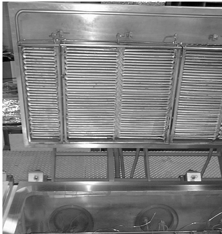
Figure 6. Ribbon heater assembly detail.
